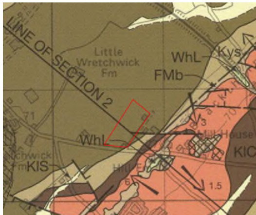
Figure 2.9: Part of BGS Geological Sheet 219 showing faults to south-east of site. (Reproduced with permission from British Geological Survey) Contains British Geological Survey materials © UKRI 2024
