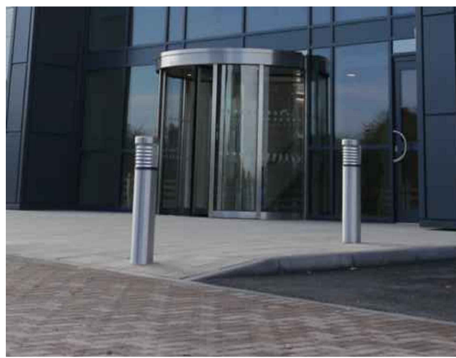
Image of illuminated brushed stainless steel bollards
