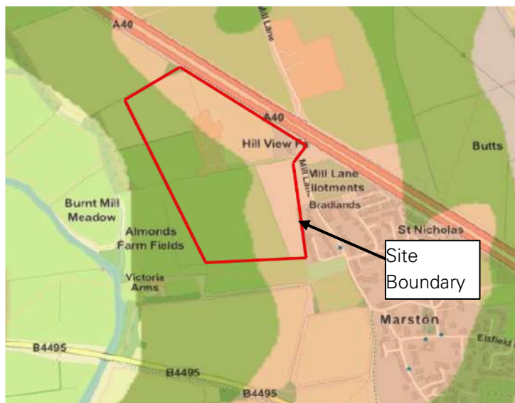
Figure 2b- Geology at the site with approximate site boundary Green = Oxford Clay Formation and West Walton Formation Pink = Oxford Clay Formation and West Walton Formation & Summertown-radley Sand and Gravel Member (British Geological Survey, 2023)
