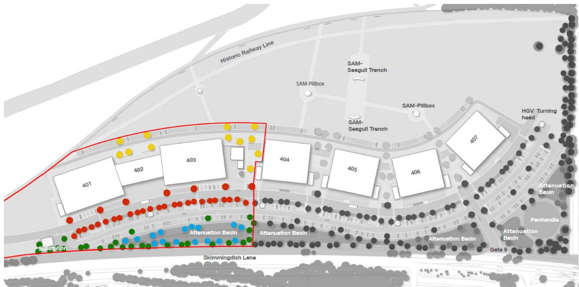
Figure 9: Extract from the DAS showing the proposed planting strategy and SuDS features.
