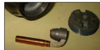
Left: baseplate and detonator removed
