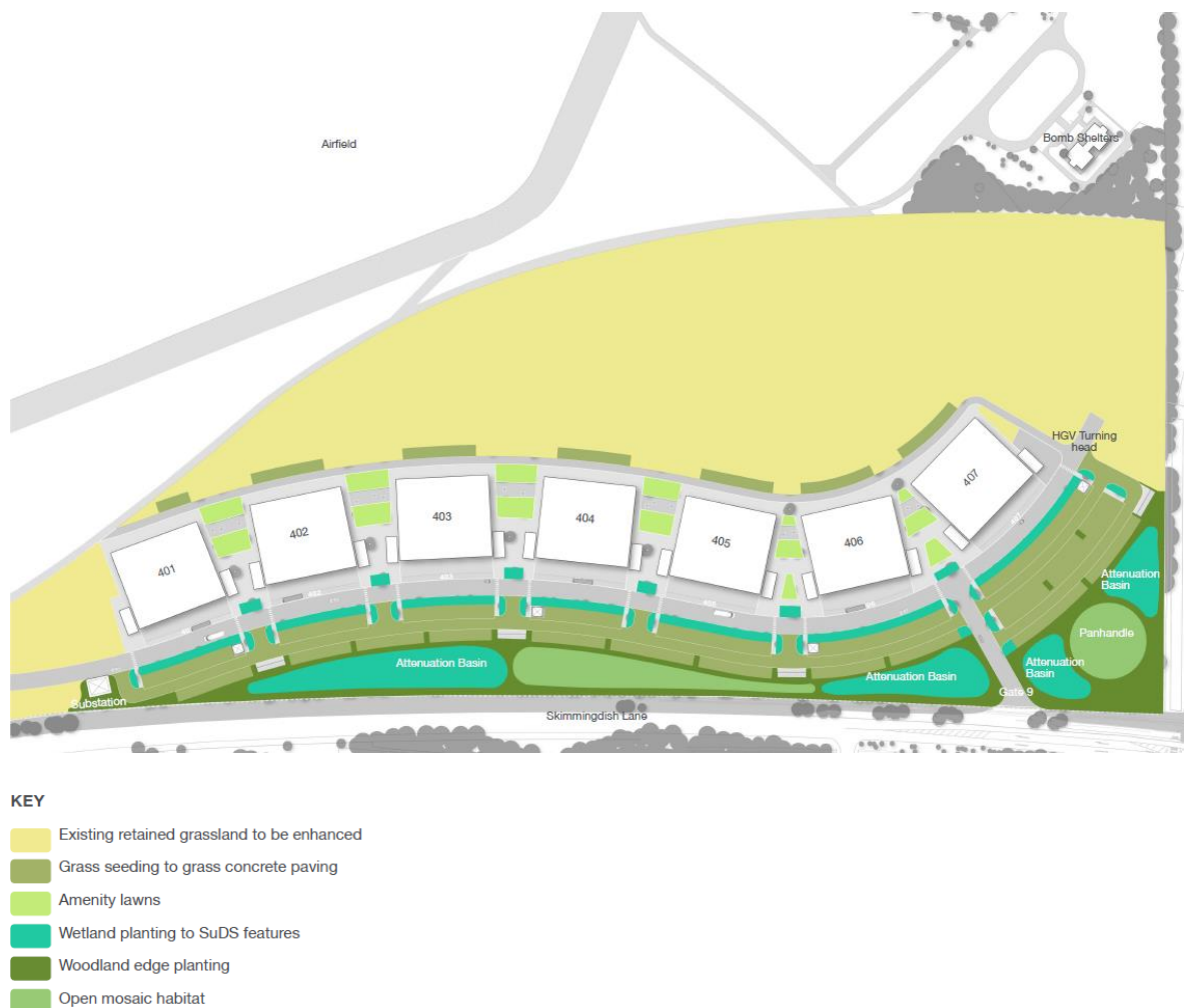
Figure 8: Extract from the DAS showing the proposed planting strategy and SuDS features.
