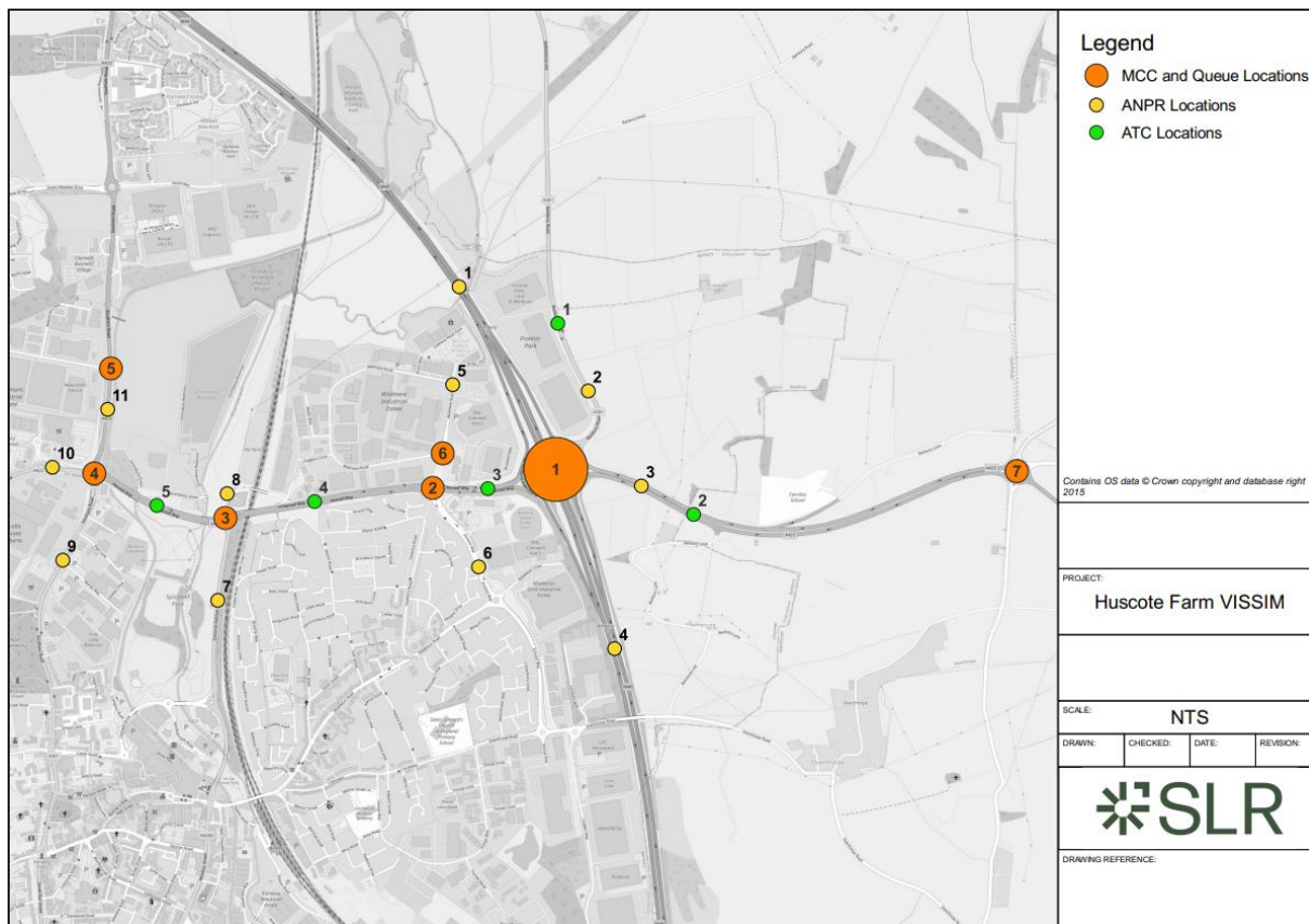
Figure 2: MCC, ANPR, and ATC Locations
