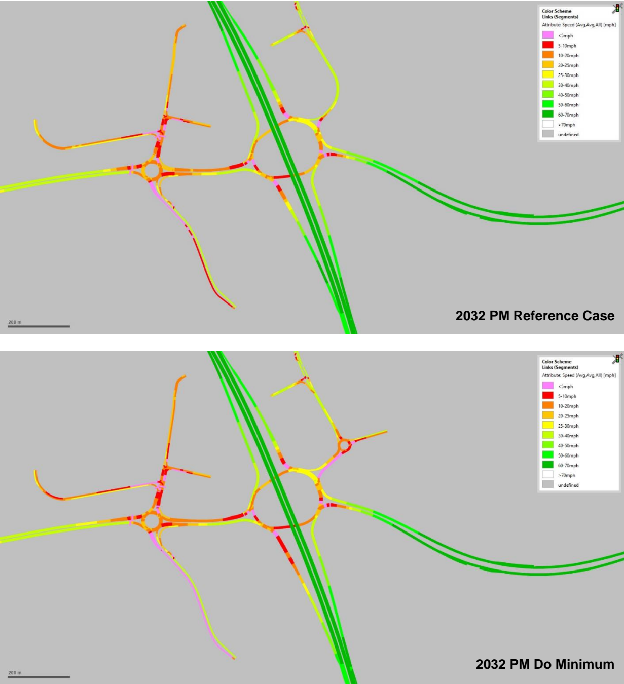
Figure 7-5 Average Speed Results – 2032 PM Reference case (top) and 2032 PM Do Minimum (bottom)
