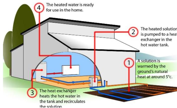
**Figure 8: Ground Source Heat Pump system diagram**
