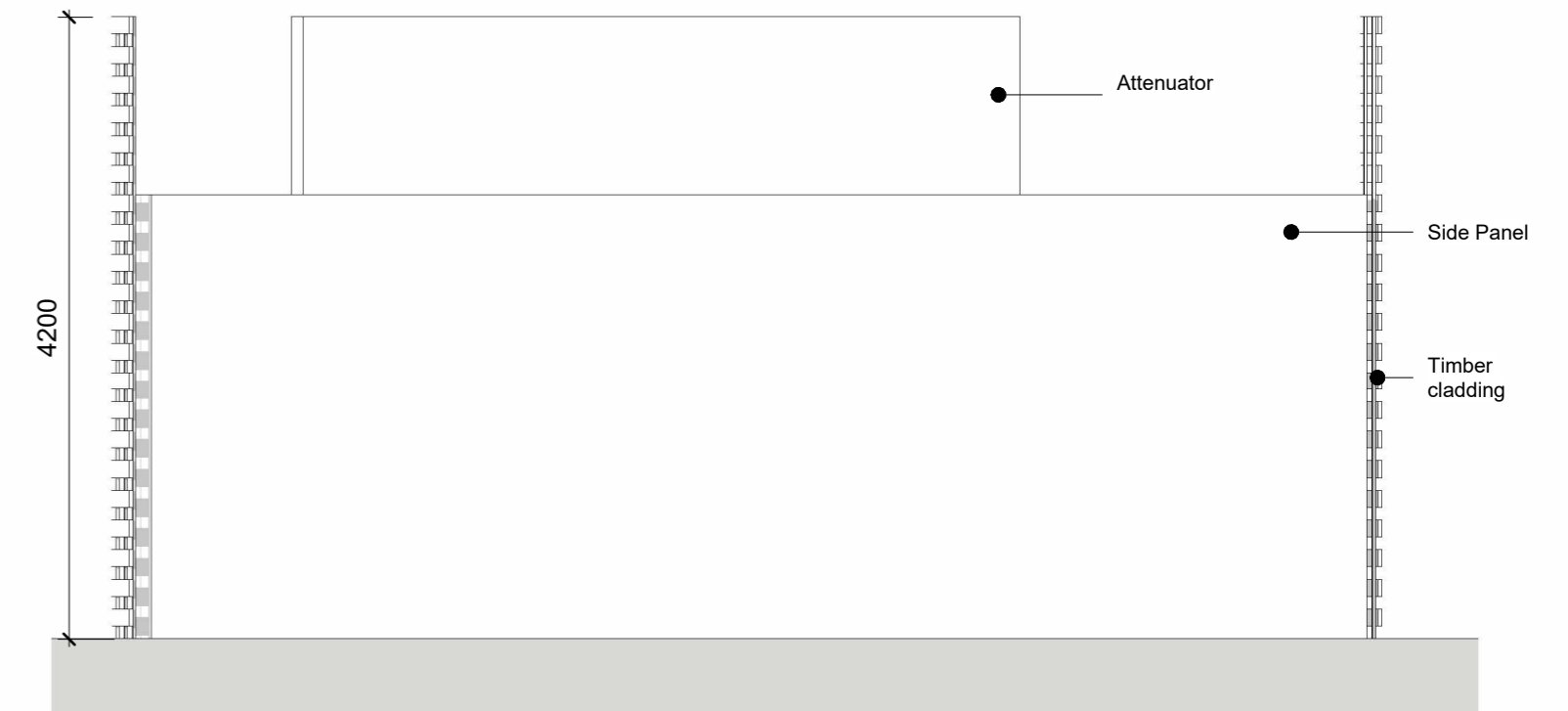
5 Elevation D-Acoustic enclosure1 1 : 50
