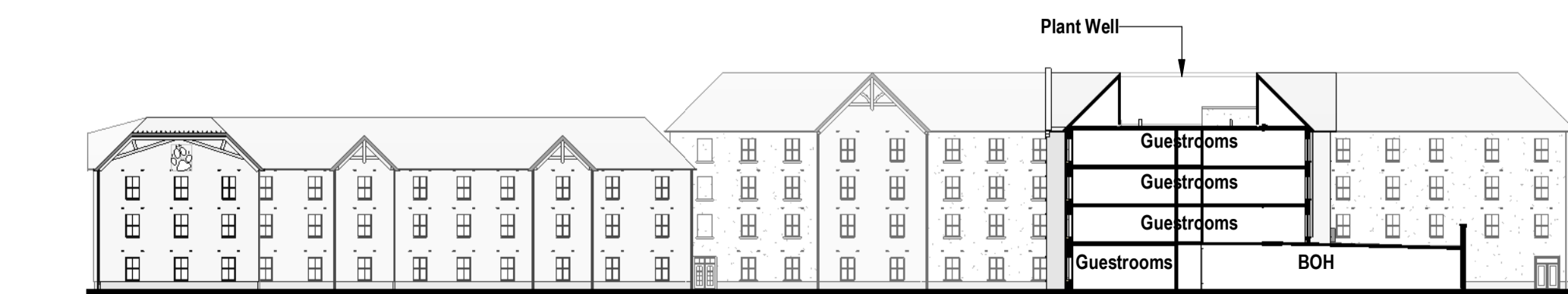
NW3 North West Elevation 3 1:500
