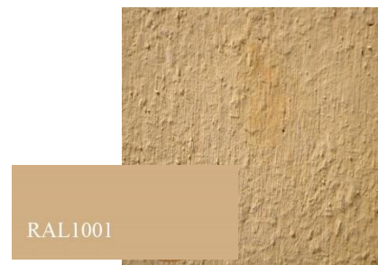
Figure 3. Clay-lime render, textured finish in yellow ochre (RAL 1001)
