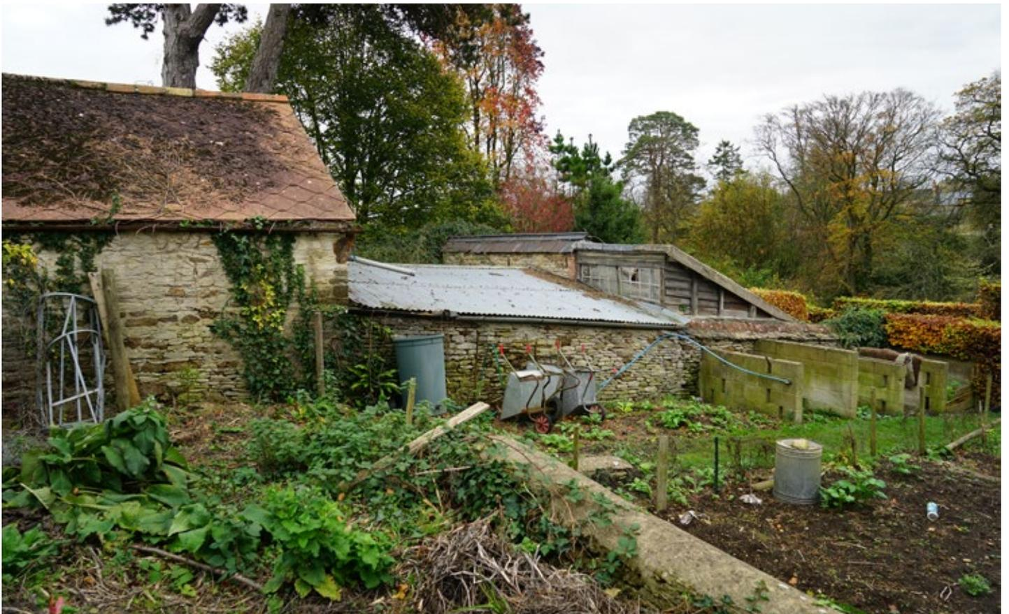
View from the west of the end of the post 1954 stable range, the corrugated metal roof of the post 1973 workshop with the rear wall of the greenhouse and attached shed infill beyond. The corrugated roof structure and supporting wall proposed to be replaced with glazed structure providing a garden lounge and access point to the approved pool. Shed to be re-conditioned and adapted to second shower and change room and the greenhouse restored
