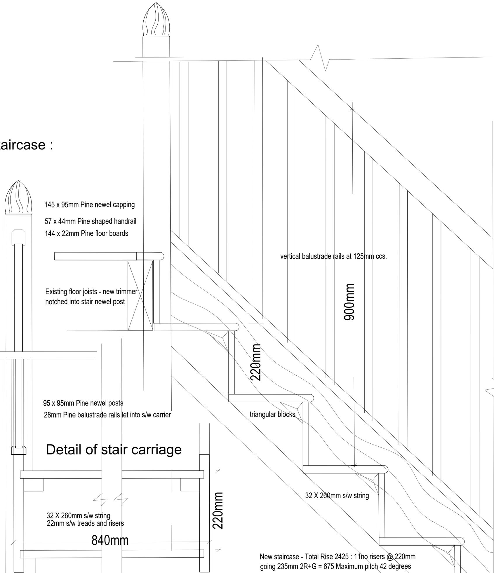
New staircase - Total Rise 2425 : 11no risers @ 220mm going 235mm 2R+G = 675 Maximum pitch 42 degrees
