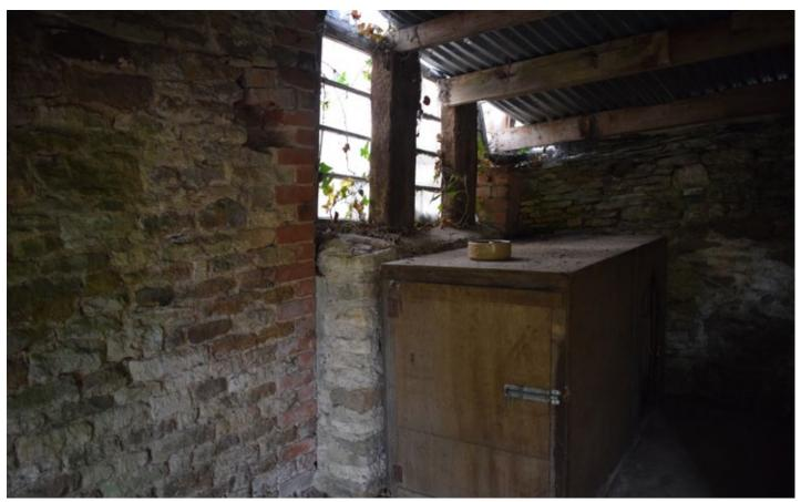
Inside the workshop showing the rear wall of the greenhouse, timber posts supporting the corrugated metal roof of the workshop and the wall to the garden beyond. Access formed into the western end of the green house and shed to form a second shower and change room
