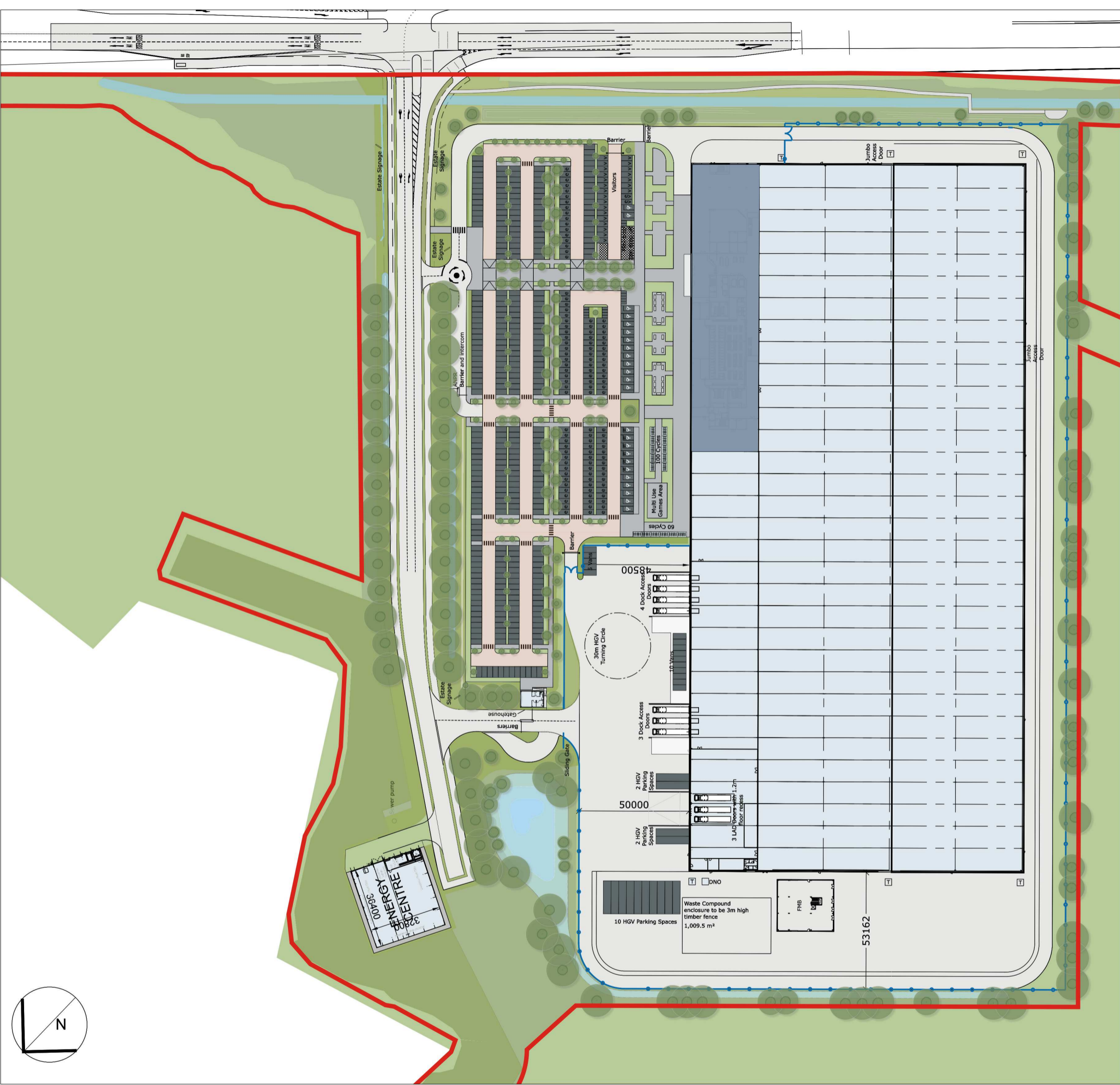
Block paving charcoal colour to pedestrian routes. Permeable paving as part of the SuDS strategy in accordance with engineers drawing : Proposed Drainage Layout T/20/2407 55-01
