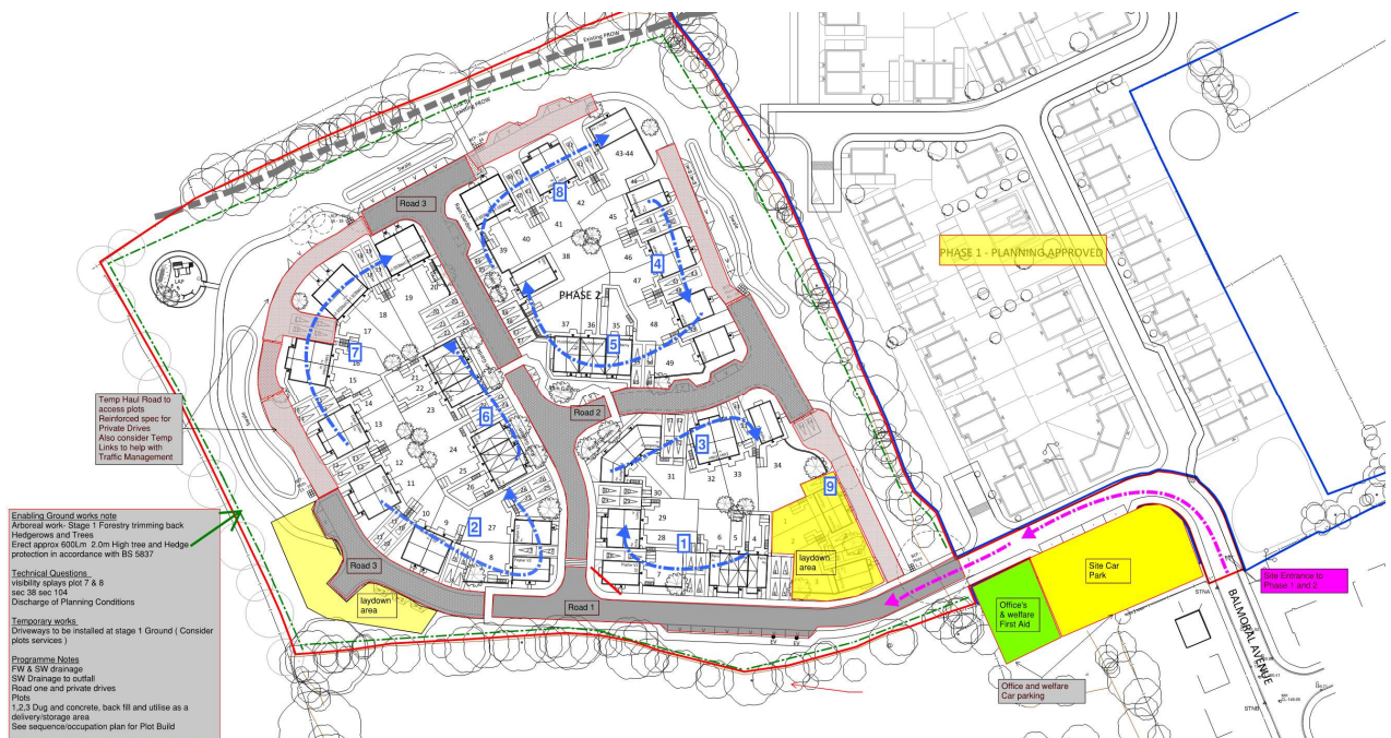
Proposed Layout and Logistics of Build Figure 2: Extract Site Compound and site Traffic Management Plan
