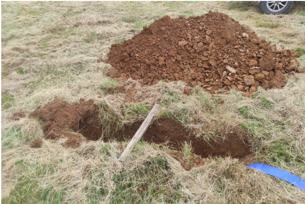
Photograph of arisings from trial pit SA4.
