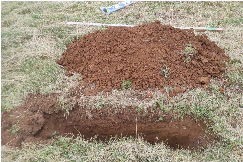
Photograph of arisings from trial pit SA2.
