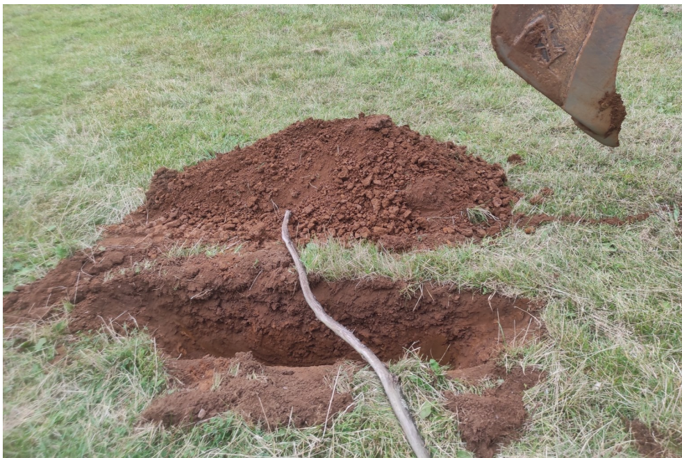
Photograph of arisings from trial pit SA8.
