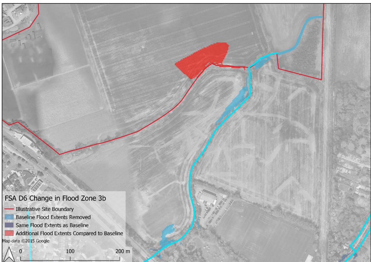
Figure 4-14 Change in Flood Extents for FSA D6 1 in 30 year, with the extent of the Ordinary Watercourse removed from the flood extents manually added to the model outputs.
