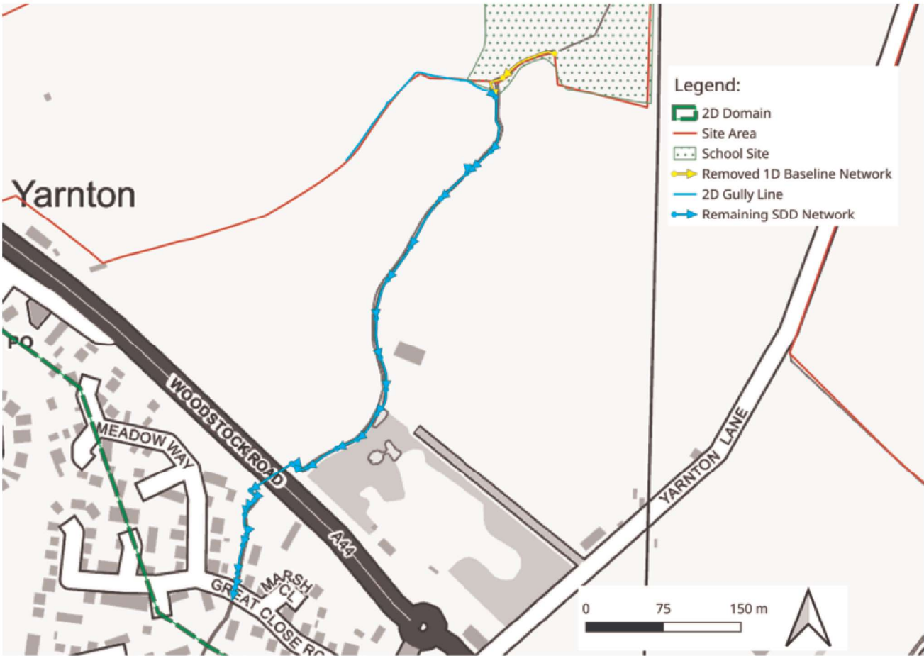
Figure 2.1: Plan showing changes between the baseline channel schematisation and the proposed condition.
