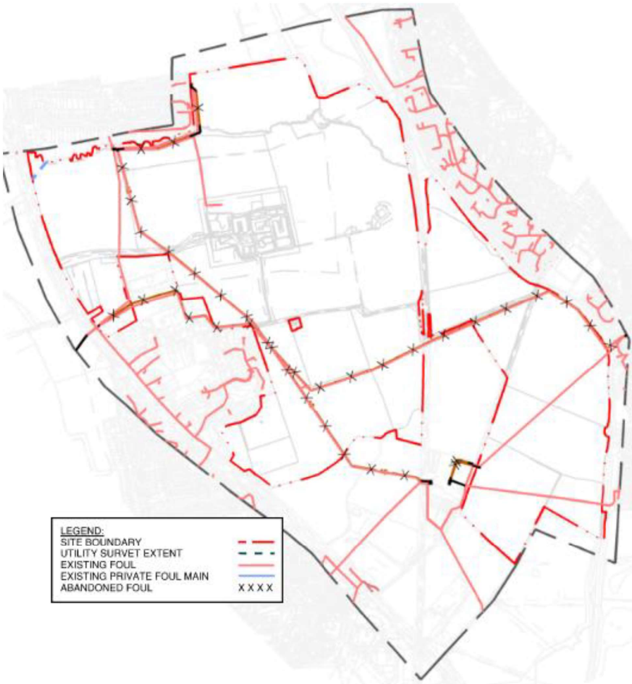
Figure 3—2 – Existing Foul Water Layout
