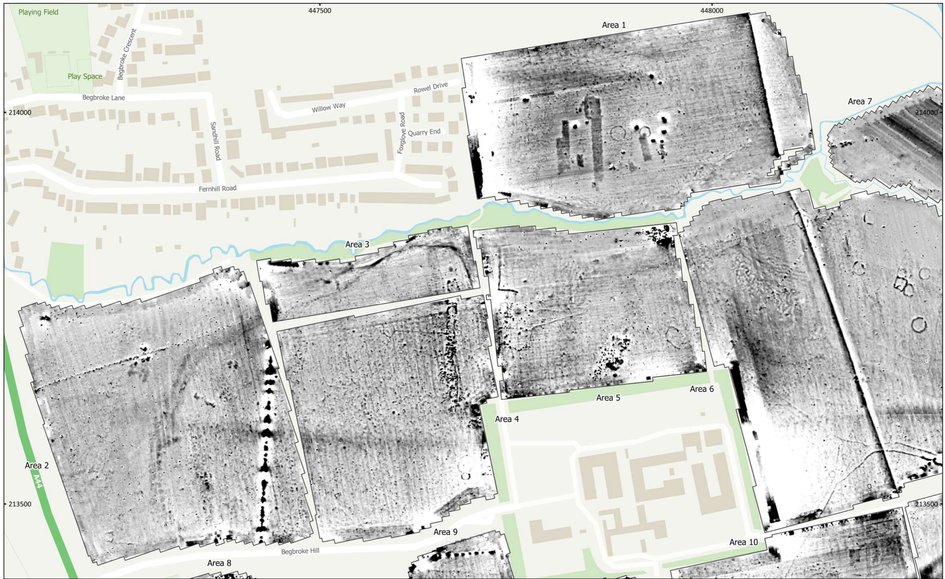
MSSP1306 - Begbroke, Oxfordshire Figure 13 - Magnetic Total Field (Lower Sensor) (Overview) (Northwest Area) 1:3,000 @ A3 Copyright Magnitude Surveys Ltd 2022 Contains Ordnance Survey data © Crown Copyright and database right 2022
