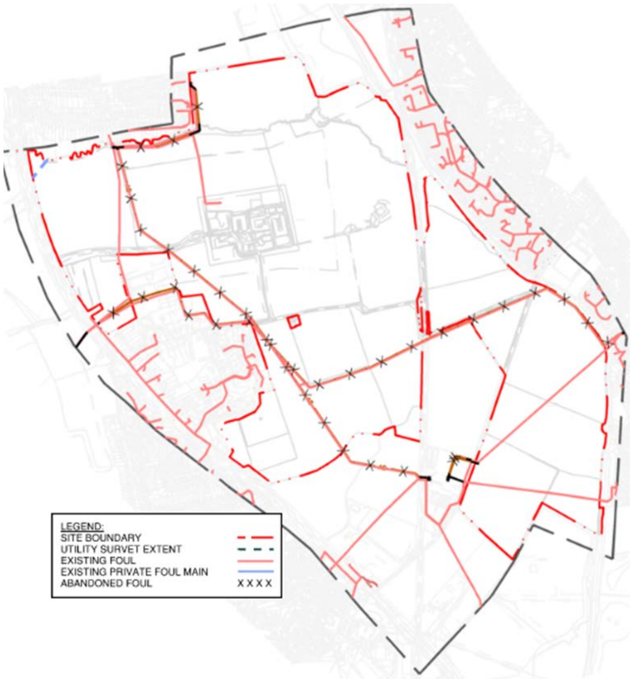
Figure 16.5: Existing Foul Water Infrastructure Layout
