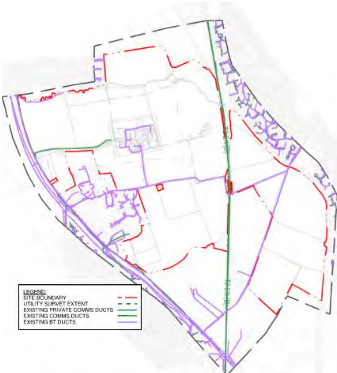
Figure 3—4 Existing Openreach Network
