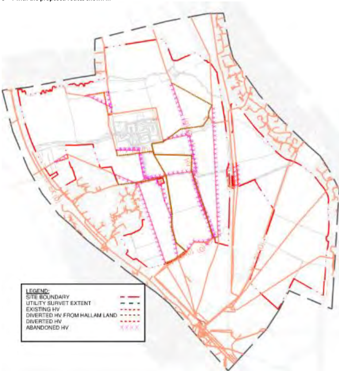
Figure 5—1. SSE have been engaged with an application for diversion. Correspondence has been received (Appendix B) confirming the below diversion routes and advising that a formal quote can be expected on the 20 th of June 2023.
