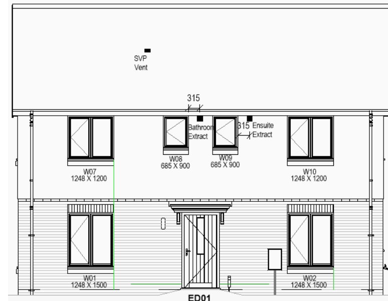
Figure 1. Marlborough House type – Front Elevation
