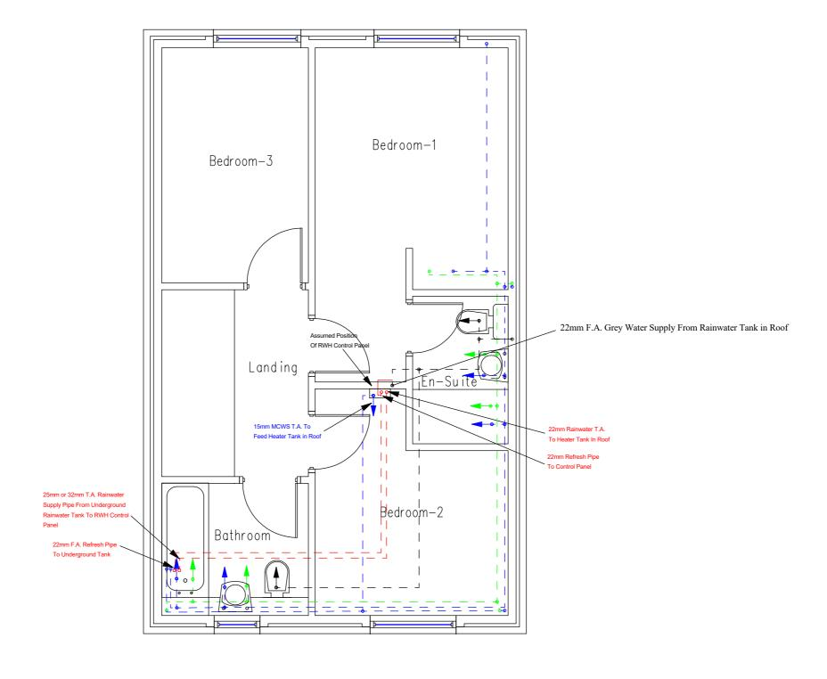
ALL HOT & COLD PLUMBING PIPEWORK (EXCLUDING MDPE) MUST BE 15mm UNLESS STATED OTHERWISE. THIS IS TO ENSURE HOT WATER RESPONSE TIMES MEET BUILDING REGULATIONS.
