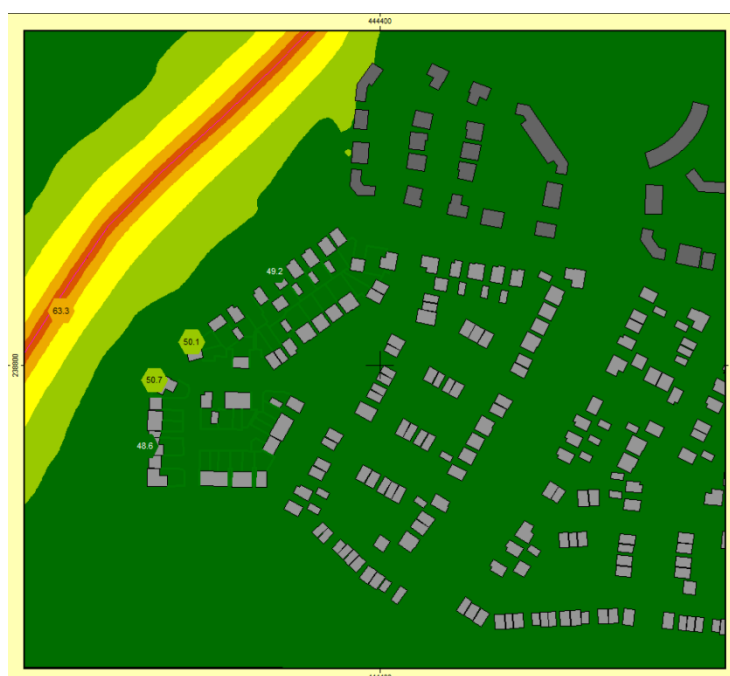
Figure 5 - Noise contour plot showing the propagation of sound across the site during the night-time
