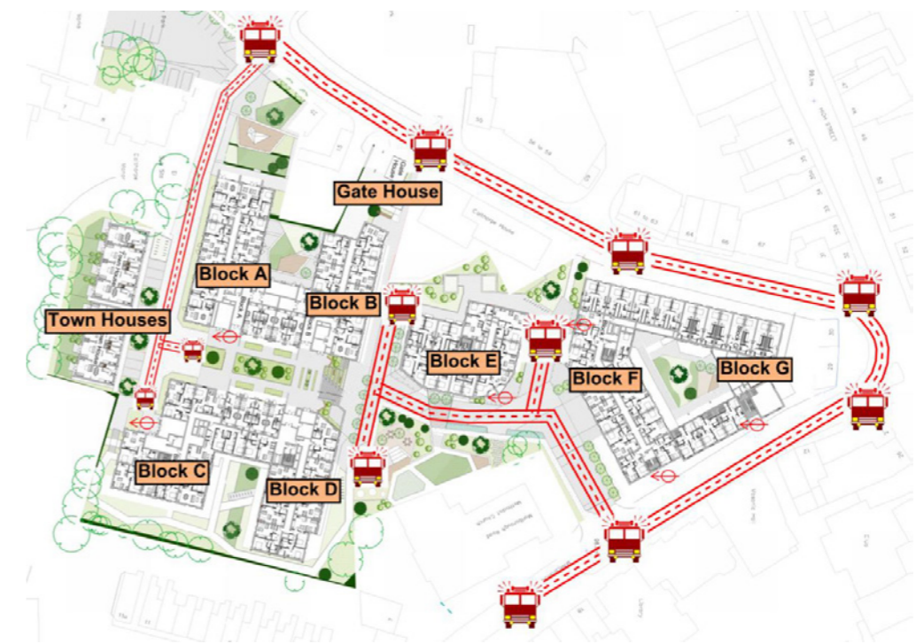
Upper Ground Floor Site Fire Access - Helios
