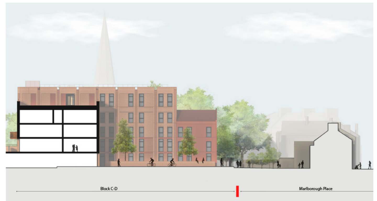
Section through Block C / D showing 4 storeys plus lower ground to centre of site - stepping down in height to 3 storeys adjacent to Marlborough Place
