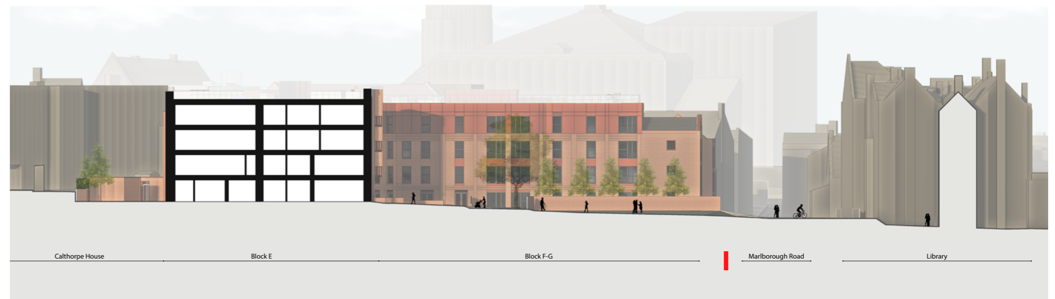
Section through Block E showing 3/4 storeys F/G to centre of site - comparable with Calthorpe House and reduced scale to Library
