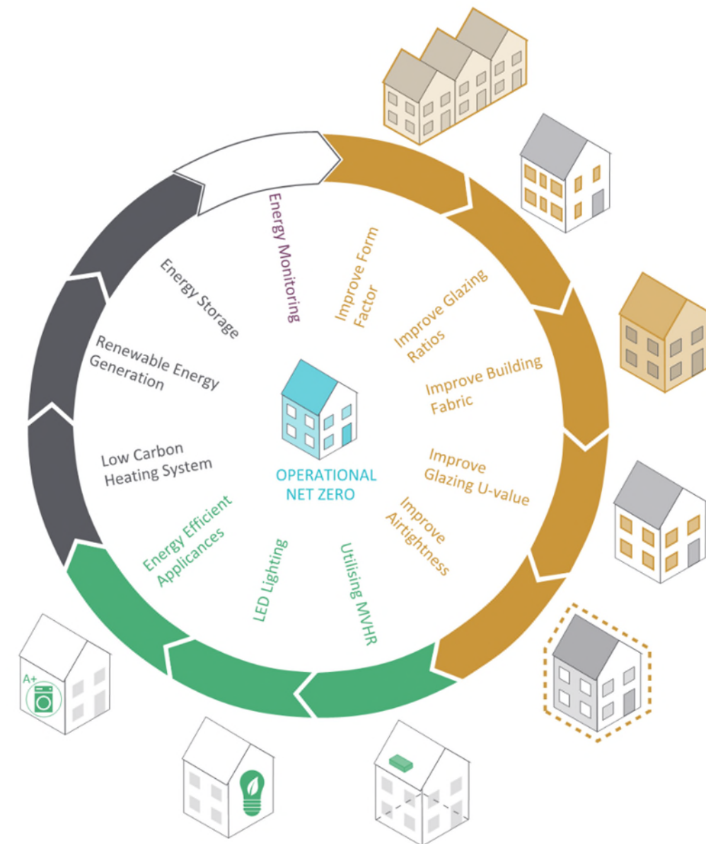
Figure 5 – Energy efficiency measures towards operational net zero
