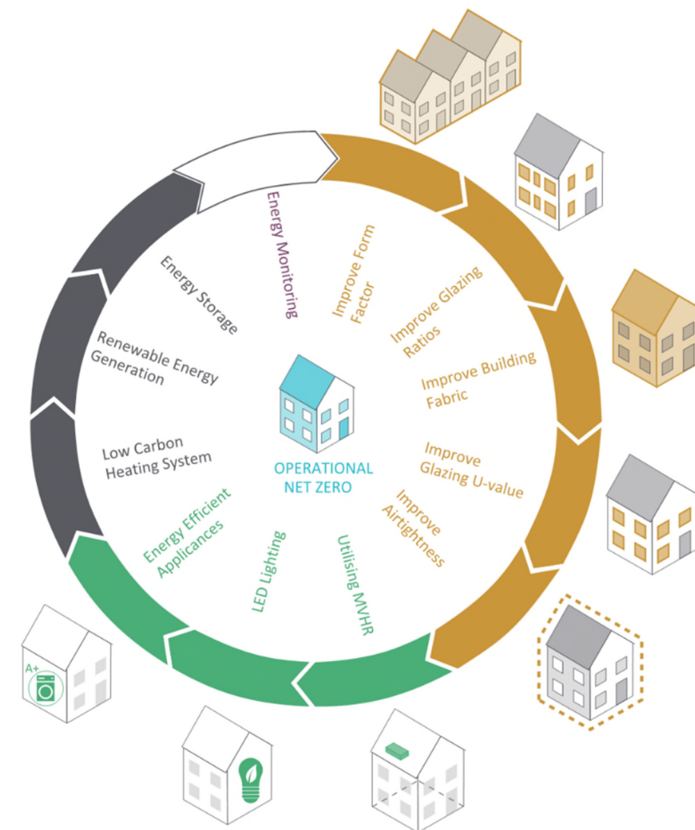
Figure 6 – Energy efficiency measures towards operational net zero
