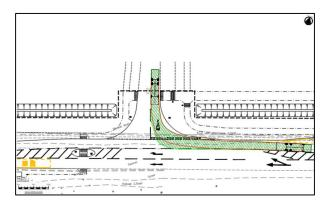
From the vehicle swept path analysis provided as part of the scheme submission, it is evident that larger service/refuse vehicle cannot turn left from the site without encroaching onto the right turn lane. Insufficient carriageway widths to accommodate long wheel based vehicular turning movements may increase the risk of vehicle on vehicle side impact/sideswipe type collisions.
