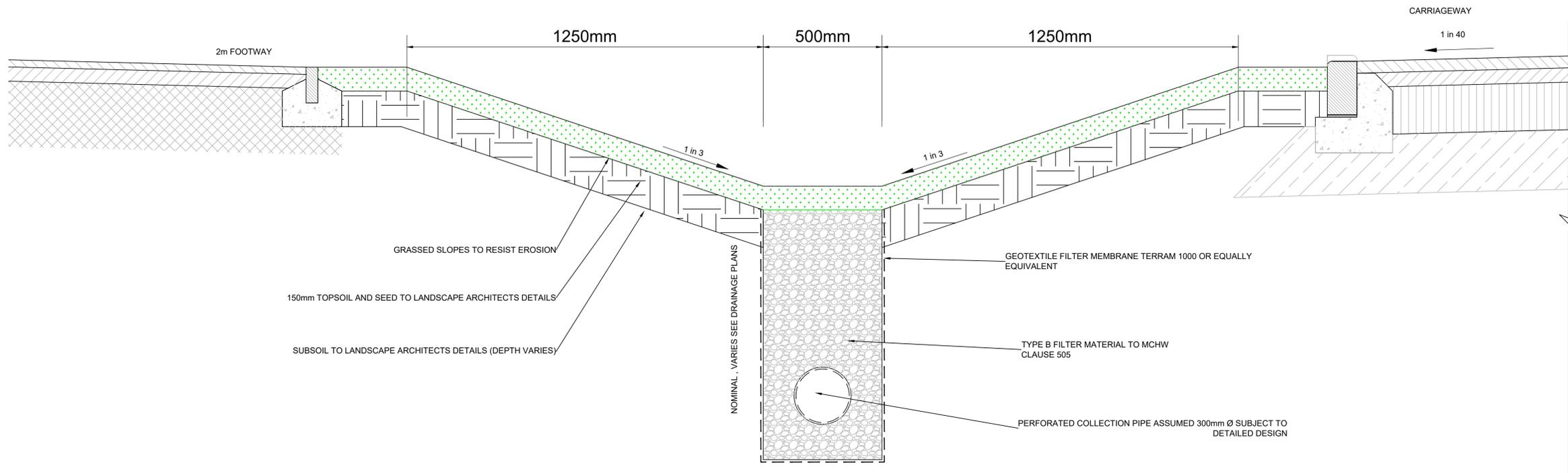
TYPICAL UNDERDRAINED SECONDARY SWALE CONSTRUCTION
