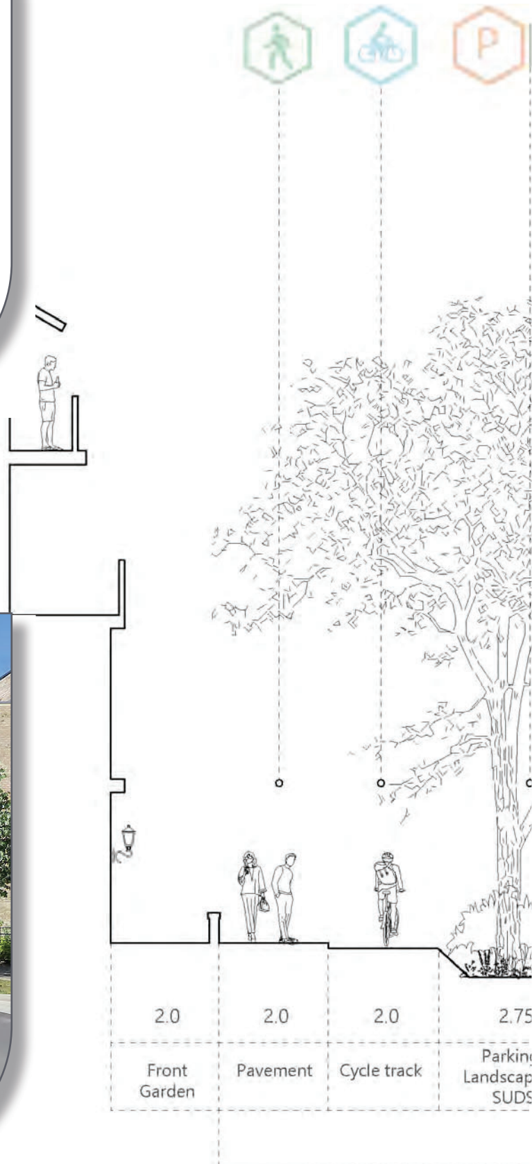
Figure 37 Primary Street Section
