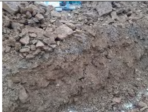
28.04.21 – Natural strata of limestone gravel in clays soil (weathered bedrock) within trench confirming limited extend of area impacted by black gravel
