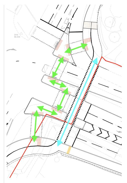
The design is a modest improvement over the initial concept in that the pedestrian and cycle crossings have been decoupled. However:
