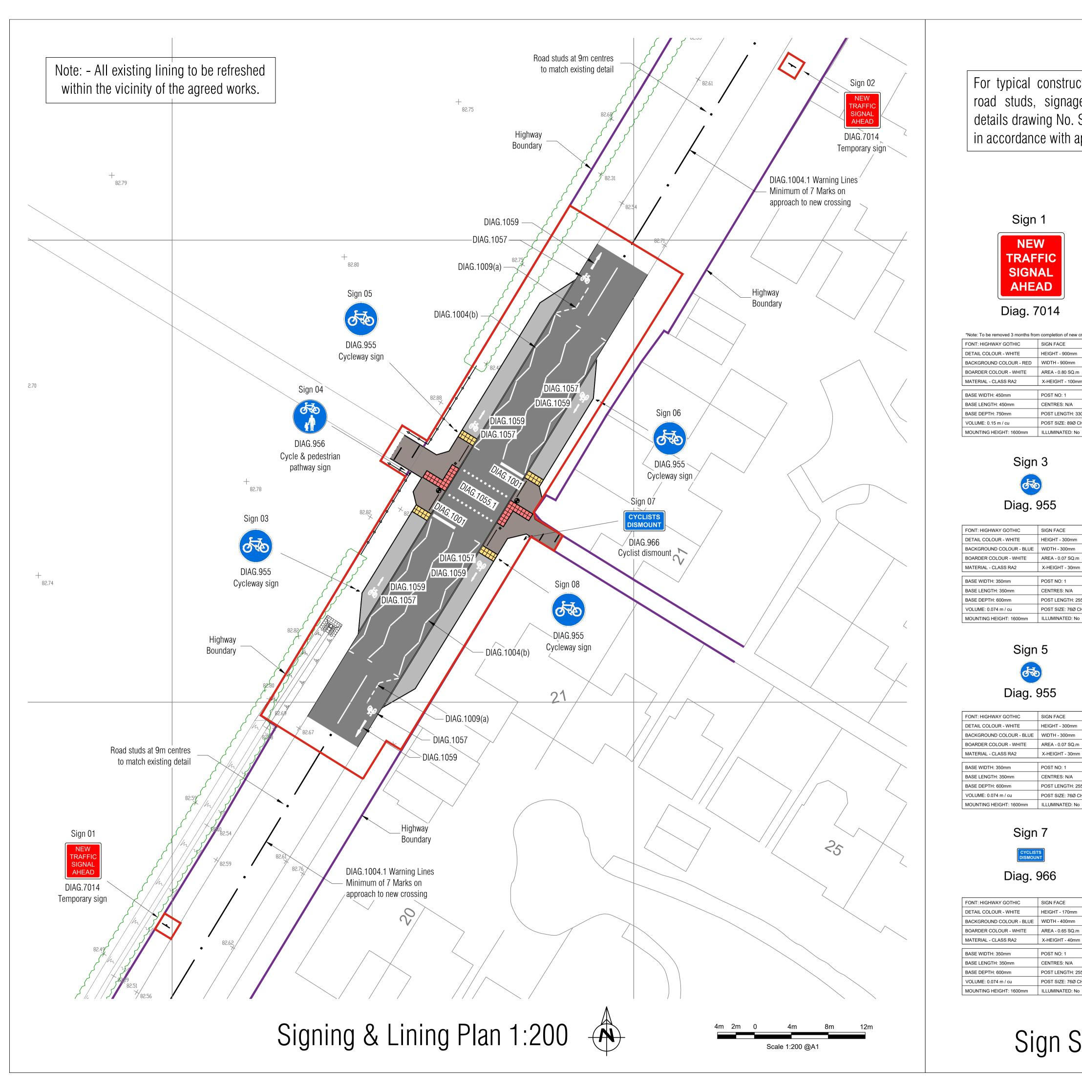
For typical construction details of sign post bases, road studs, signage notes and lining notes, see details drawing No. S1209-S278-06. All details to be in accordance with approved OCC Standard details.
