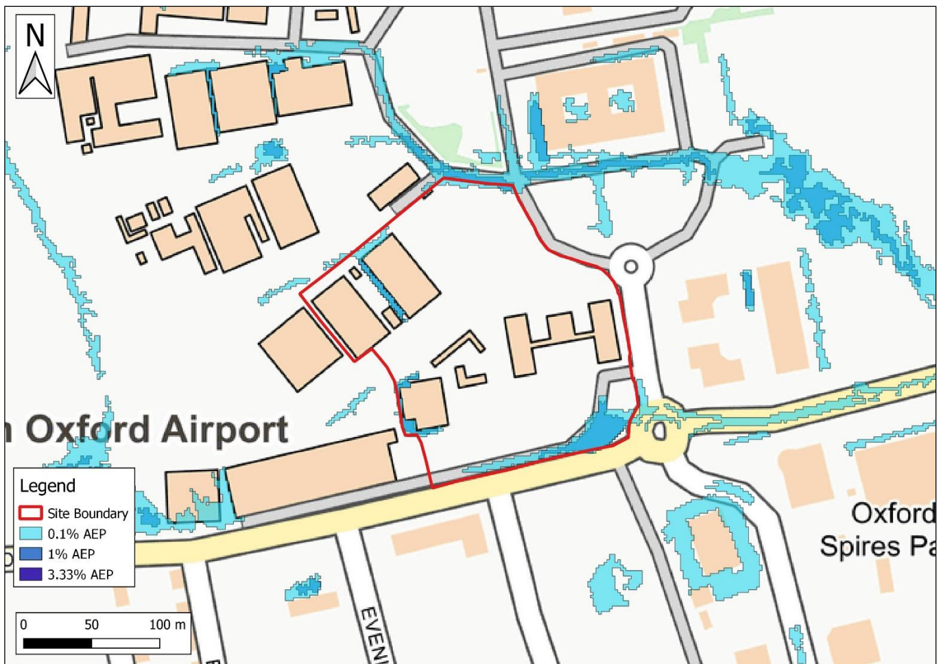
Figure 4-3: Risk of flooding from surface water mapping
