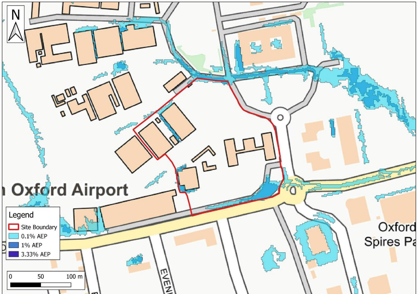
Figure 4-3: Risk of flooding from surface water mapping
