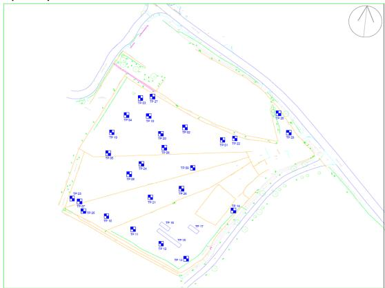
In trial trench TP15, rare fragments of Asbestos roof tile (ACM) were observed. However 3No. tubs of soil matrix were submitted to analysis for asbestos at depths of 0.50m, 0.70m and 0.90m bgl from various lengths along the pit extending in a south-easterly direction. Asbestos fibres were not recorded.
