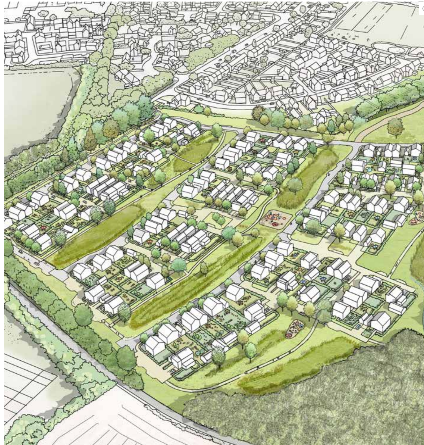
01 Indicative Aerial Sketch - illustrating buildings primarily facing east / west to minimise energy consumption.
