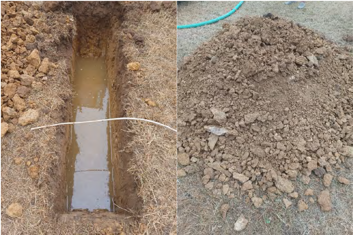
TP02 Ground Level to 1.2m bgl during Infiltration Test
