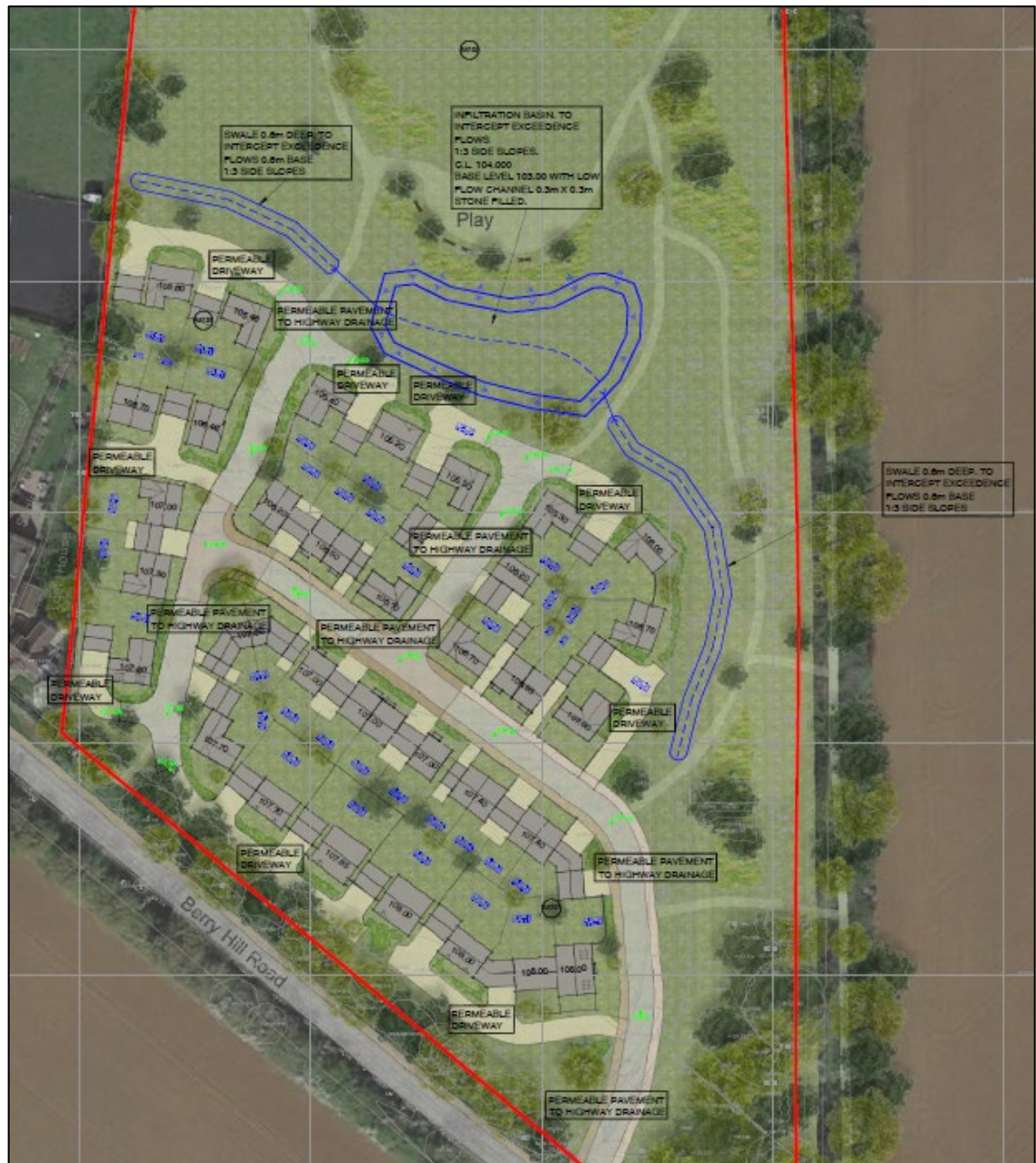
Figure 1.3.2: Ironside Farrar Preliminary Drainage Layout (Drawing No: 30394/102)
