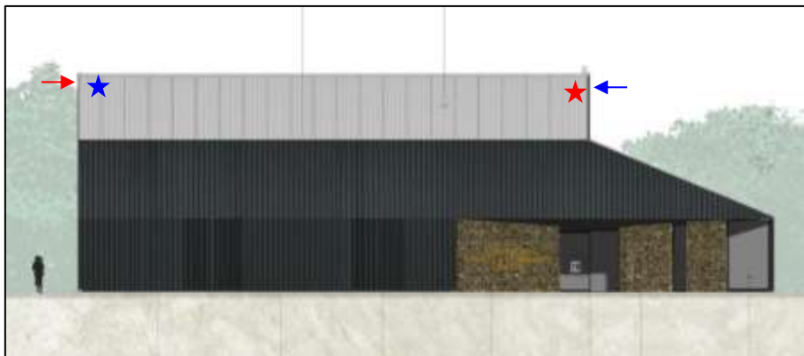
Figure 4b. Location of bat tubes and swift boxes on the south elevation of the proposed community centre building (blue stars=bat tubes, red stars=swift boxes, blue arrow=bat tube on adjacent corner, red arrow=swift box on adjacent corner)
