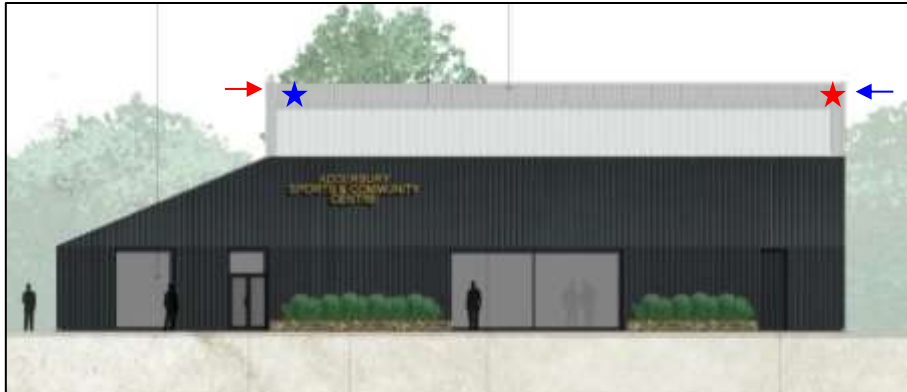
Figure 4b. Location of bat tubes and swift boxes on the south elevation of the proposed community centre building (blue stars=bat tubes, red stars=swift boxes, blue arrow=bat tube on adjacent corner, red arrow=swift box on adjacent corner)
