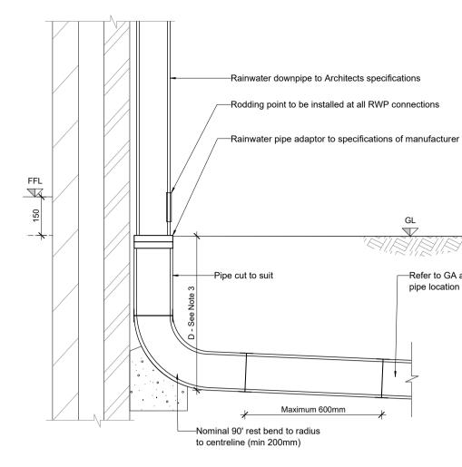
8251 - External Rainwater Pipe Connection Detail
