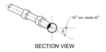
NOTES: 1. The vertical angle between the connecting pipe and the horizontal should be greater than 0° and not more than 60°. Where the connection is being made to a sewer with a nominal internal diameter of 300 mm or less, connections should be made using 45° angle, or 90° angle, curved square junctions. 3. Connections made with junction fittings should be made by cutting the existing pipe, inserting the junction fitting and jointing with flexible repair couplings or slip couplers.
