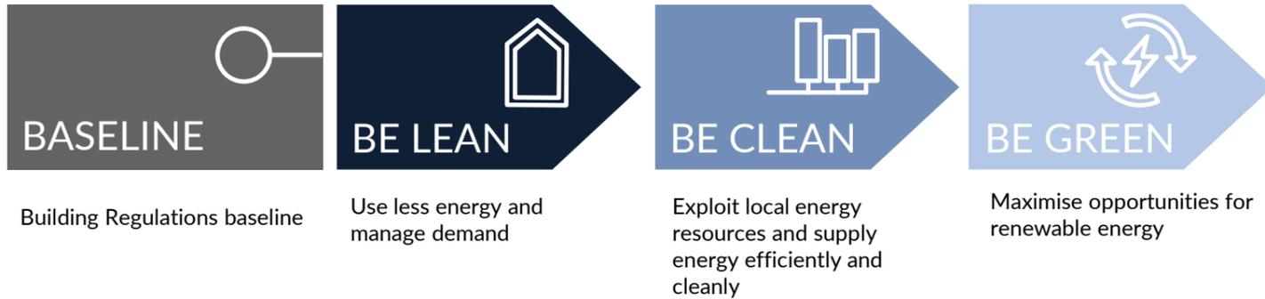
As this hierarchy demonstrates, designing out energy use in the first instance is weighted more favourably than the generation of low-carbon or renewable energy to offset unnecessary demand. Applied to this development, the 'fabric first' approach concentrates efforts on:
