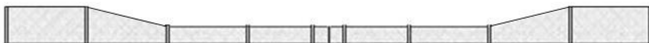
East Side Elevation – Length 35 metres – Height ranging from 2 metres down to 0.9 metres
