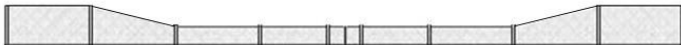
West Side Elevation – Length 35 metres – Height ranging from 2 metres down to 0.9 metres
