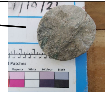
Photograph 3d: Fracture surface at 4.54 m bgl.
