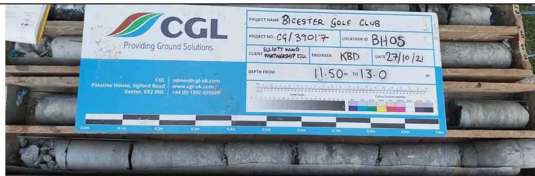
Photograph 20: Core run between 11.5 and 13.0 m bgl of mudstone and limestone of the Forest Marble Formation in BH05. Base of borehole at 13.0 m bgl.
