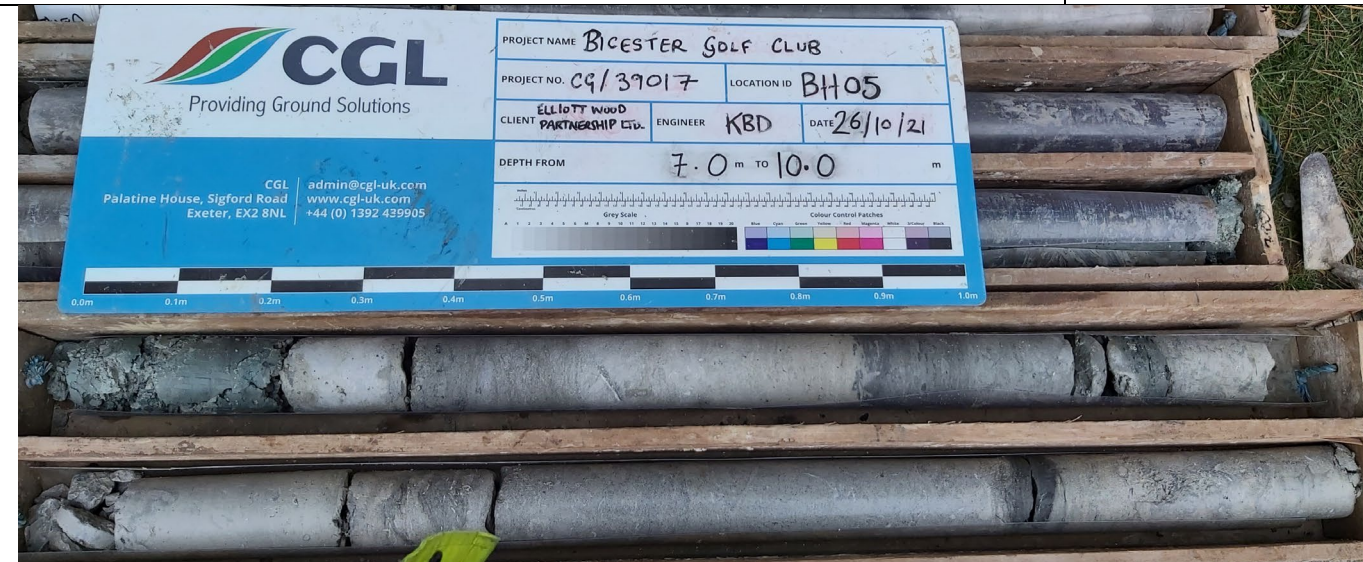
Photograph 18: Core run between 7.0 and 10.0 m bgl of mudstone and limestone of the Forest Marble Formation in BH05.
