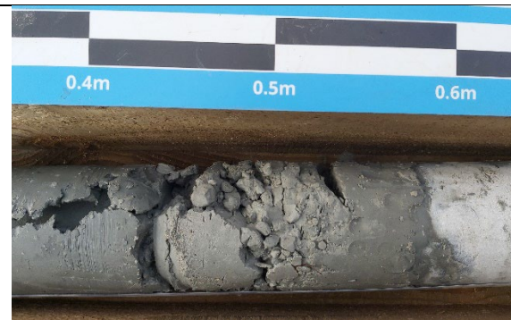
Photograph 3b: Weak mudstone recovered as gravel between 3.9 and 4.1 m bgl.
