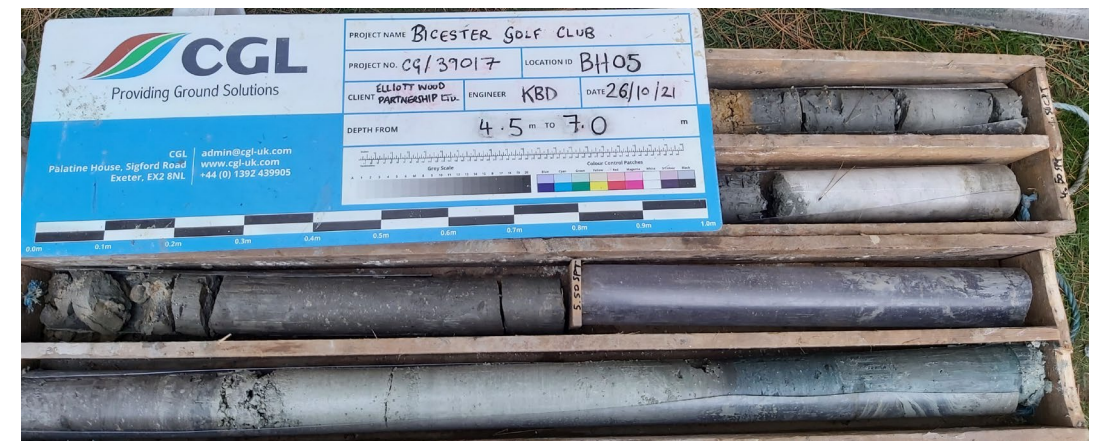
Photograph 17: Core runs between 4.5 and 7.0 m bgl of mudstone, clay, and limestone of the Forest Marble Formation in BH05.
