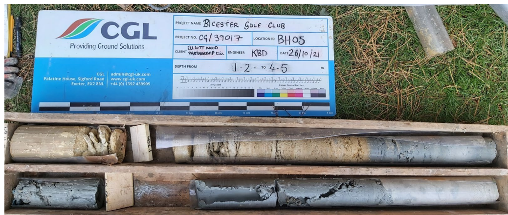
Photograph 16: Core runs between 1.2 and 4.5 m bgl of marl of the Cornbrash formation and the boundary between with the clay of the Forest Marble Formation in BH05.
