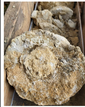
Photograph 16a: Marl between 1.2 and 1.5 m bgl.
