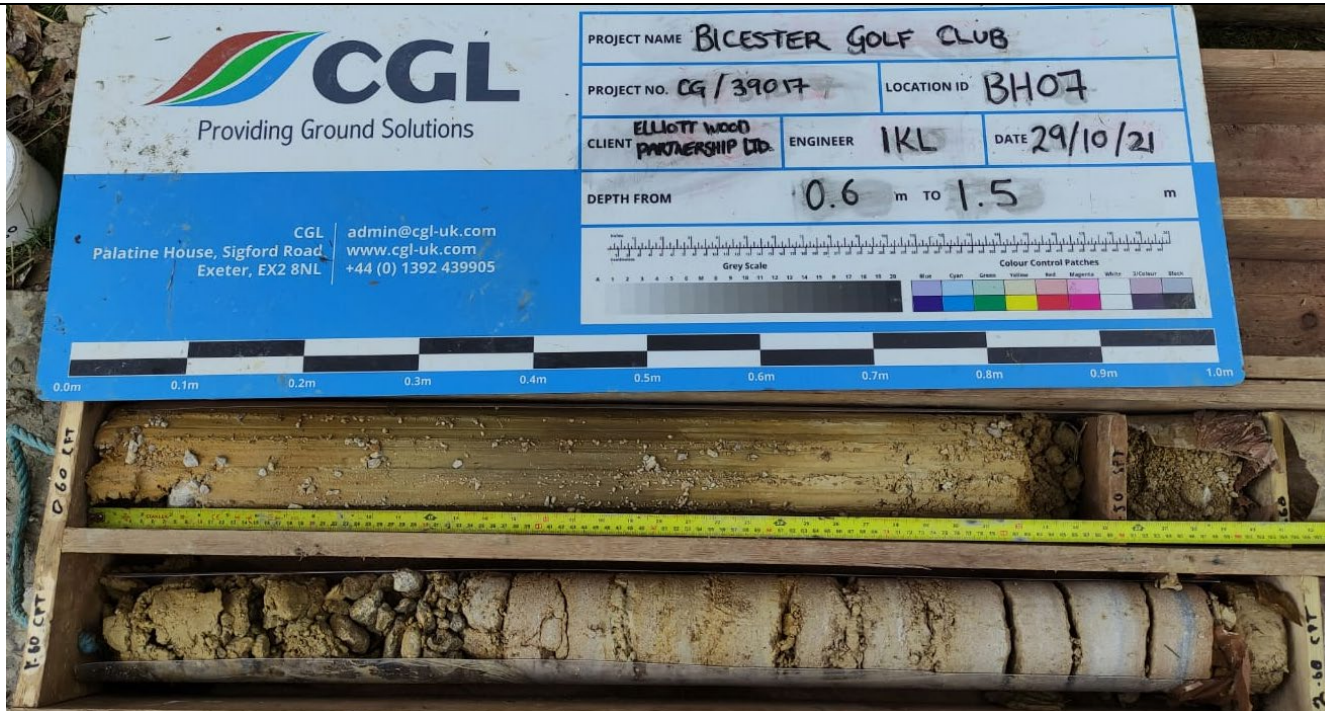
Photograph 23: Core runs between 0.6 and 2.6 m bgl of marl and limestone of the Cornbrash Formation in BH07.
