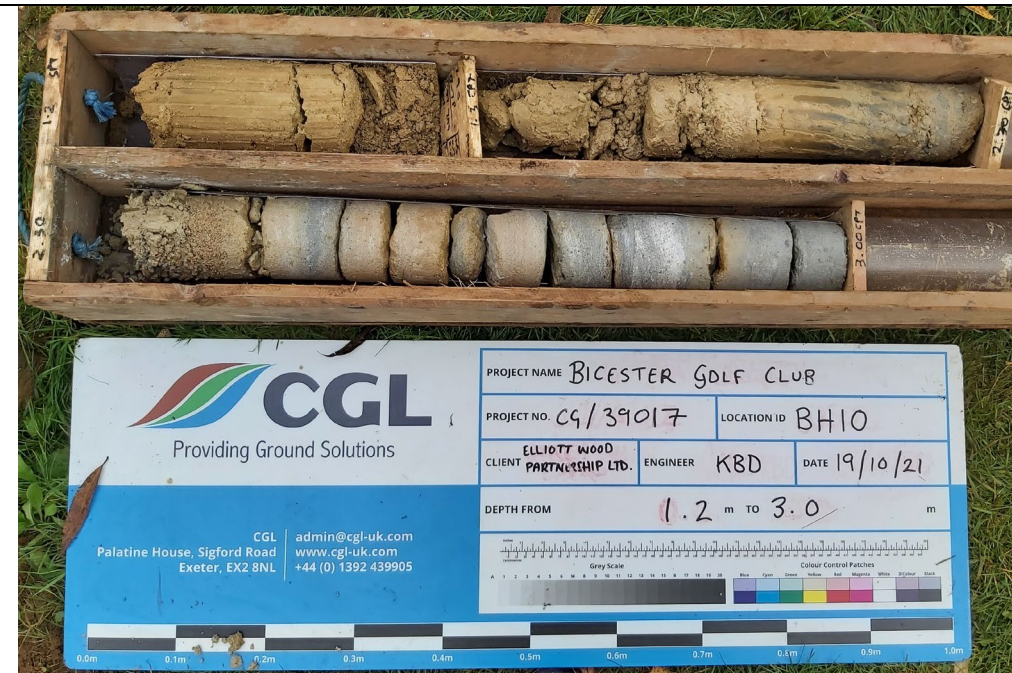
Photograph 28: Core runs the Cornbrash Formation between 1.2 – 3.0 m bgl in BH10.
