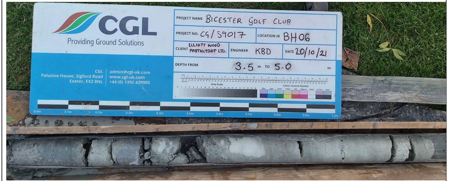
Photograph 22: Core runs between 3.5 and 5.0 m bgl of mudstone, and limestone of the Forest Marble Formation in BH06. End of borehole at 5 m bgl.
