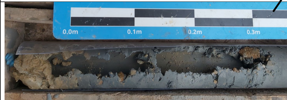
Photograph 1c: Intact light brown to pinkish orange mottled grey medium grained limestone – the base of the Cornbrash Formation. Between 2.10 and 2.55 m bgl.
