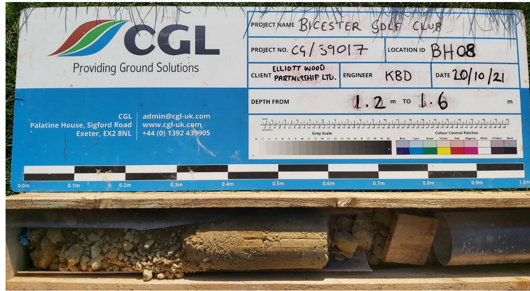
Photograph 25: Core run of sandy gravelly clay of the Cornbrash Formation between 1.2 – 1.6 m bgl in BH08.
