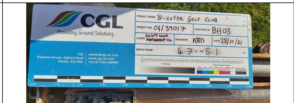
Photograph 3: Core run of dark grey mudstone between 4.70 m and 5.00 bgl.
