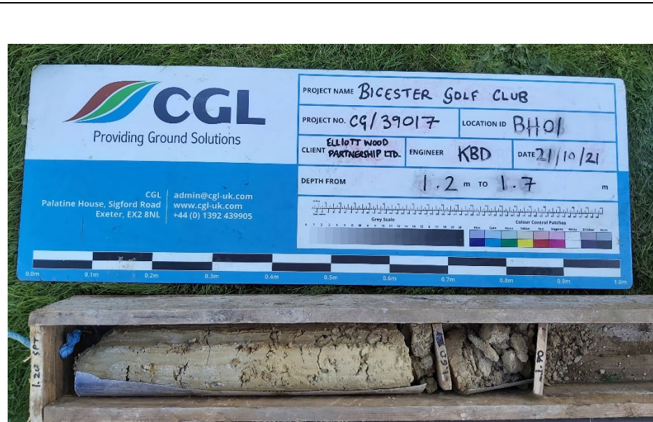
Photograph 1: Core run of sandy gravelly clay between 1.2 – 1.7 m bgl in BH01.
