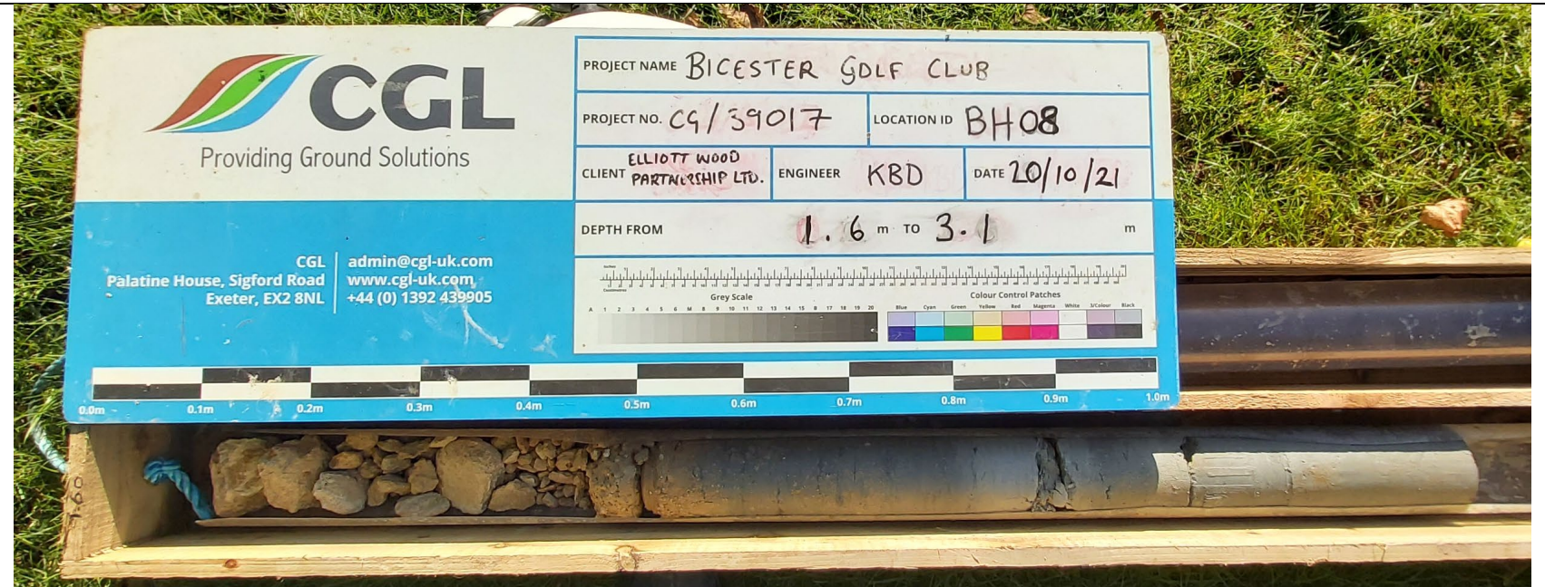
Photograph 26: Core run between 1.6 -3.1 m bgl showing the boundary between the Cornbrash Formation and the Forest Marble Formation in BH08.
