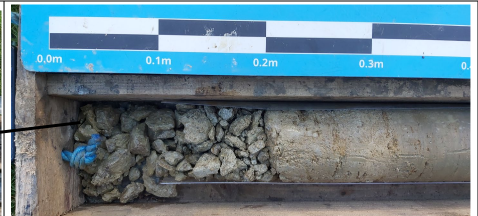
Photograph 1b: limestone recovered as gravel between 1.70 and 1.85 m bgl.
