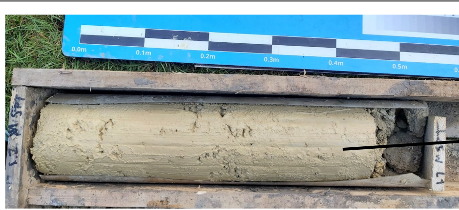
Photograph 1a: Core run between 1.2 and 1.70 m bgl of stiff slightly gravelly clay.
