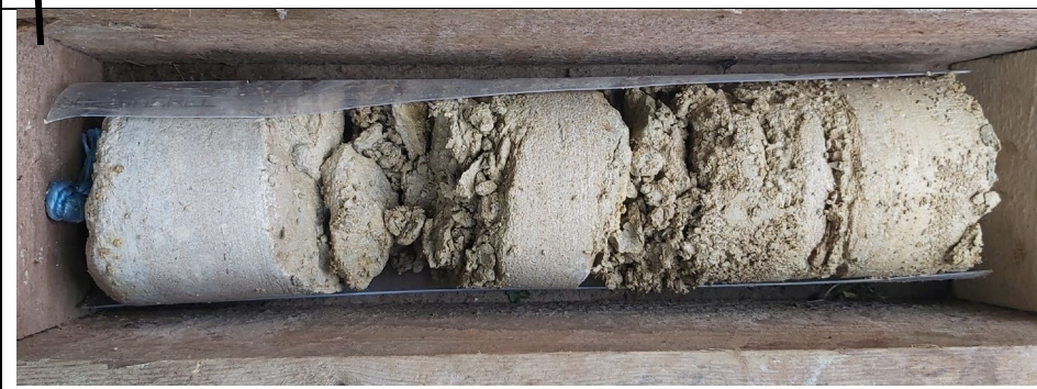
Photograph 1c: Intact light brown to pinkish orange mottled grey medium grained limestone – the base of the Cornbrash Formation. Between 2.10 and 2.55 m bgl.
