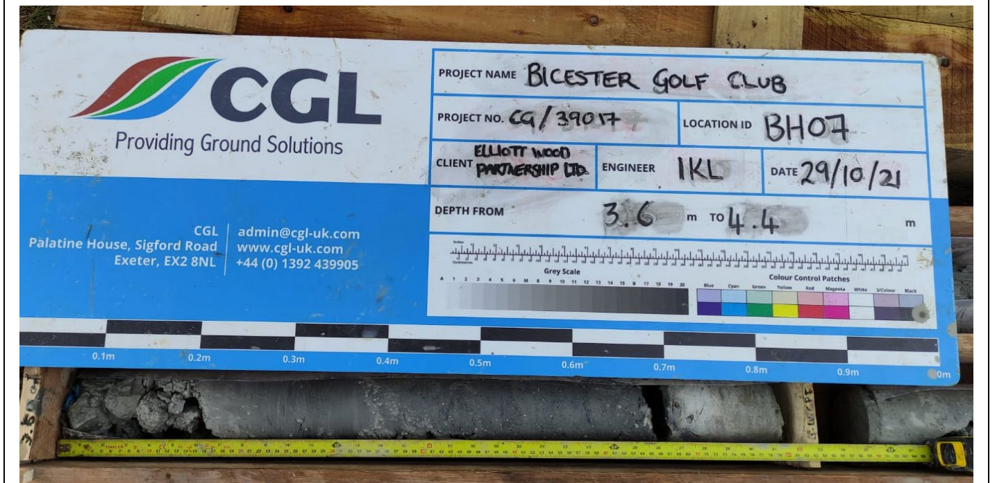
Photograph 24: Core run between 3.6 and 4.4 m bgl of mudstone and limestone of the Forest Marble Formation in BH07.
