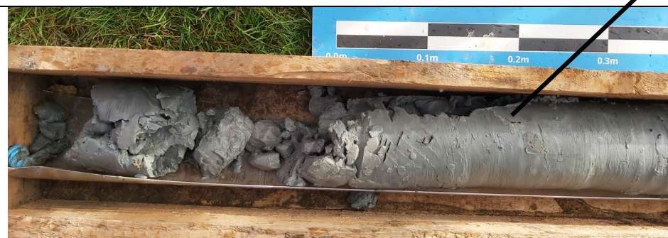
Photograph 1c: The boundary between the brown limestone of the Cornbrash Formation and the grey mudstone of the Forest Marble Formation, at ~2.0 m bgl.
