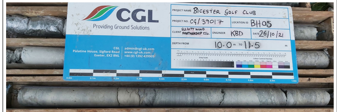
Photograph 19: Core run between 10.0 and 11.5 m bgl of mudstone and limestone of the Forest Marble Formation in BH05.
