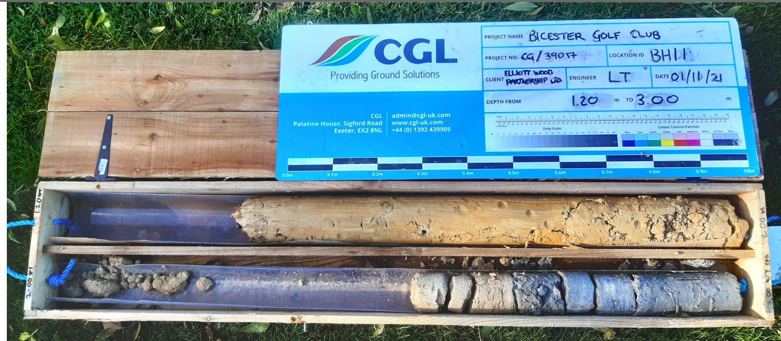
Photograph 29: Core runs between 1.2 - 3.0 m bgl in BH11.
