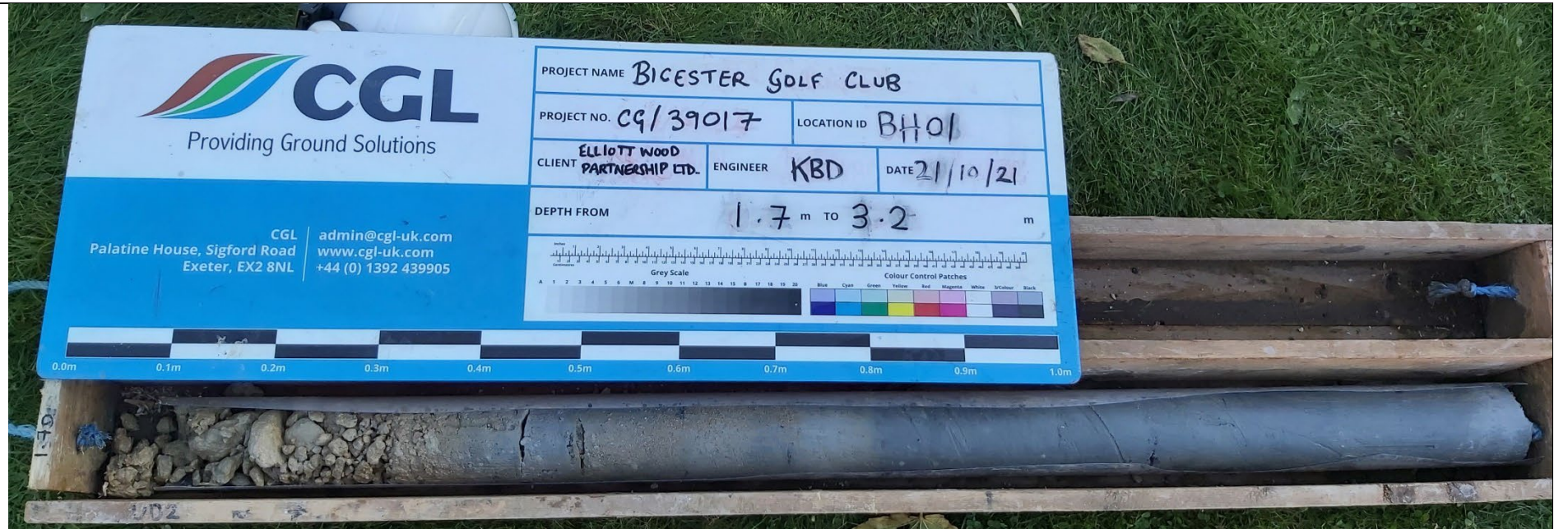
Photograph 2: Core run between 1.7 -3.2 m bgl. Clayey limestone gravel between 1.7 and 2.0, and stiff becoming very stiff dark grey clay between 2.0 and 3.2 m bgl in BH01.
