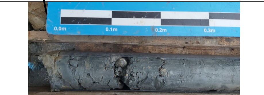
Photograph 2c: Firm slightly sandy slightly gravelly clay between 4.00 and 4.30 m bgl.
