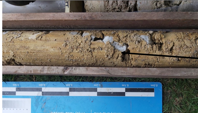
Photograph 10a: Marl as recovered - described as firm to stiff sandy gravelly clay between 0.70 and 1.5 m bgl.
