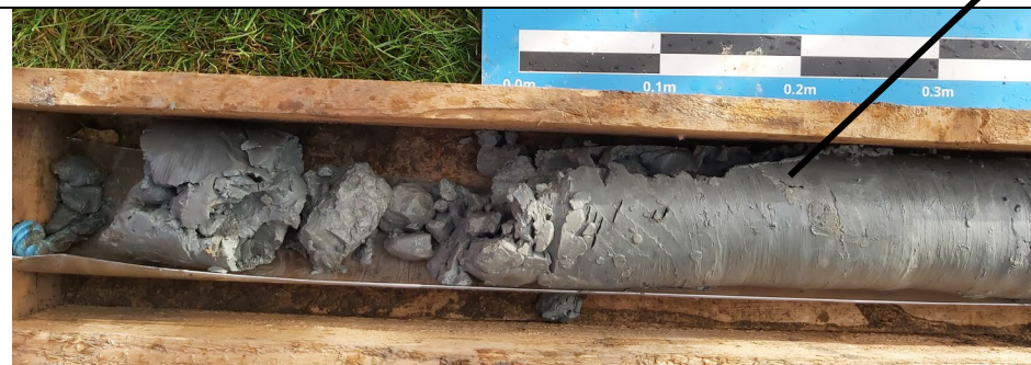
Photograph 7c: The boundary between the brown limestone of the Cornbrash Formation and the grey mudstone of the Forest Marble Formation, at ~2.0 m bgl.
