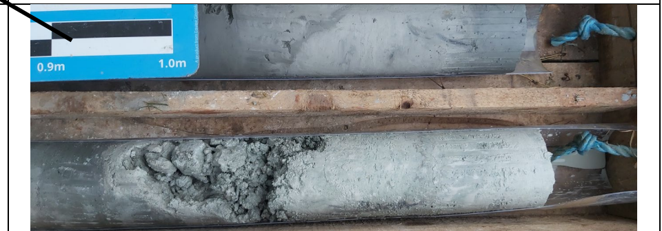
Photograph 11d: Weak greenish grey mudstone between 4.90 and 5.50 m bgl, recovered as gravel between 4.90 and 5.10 m bgl.
