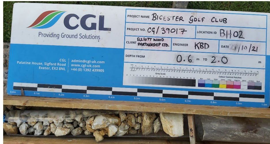
Photograph 4: Limestone gravel between 1.34 and 2.00 m bgl in BH02.
