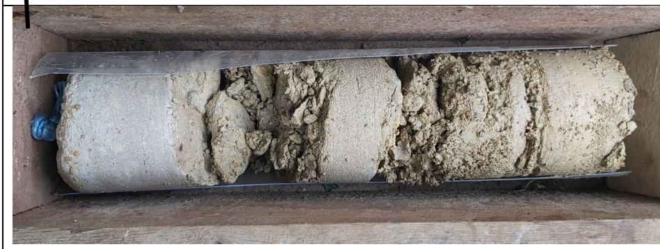
Photograph 10c: Intact light brown to pinkish orange mottled grey medium grained limestone – the base of the Cornbrash Formation. Between 2.10 and 2.55 m bgl.
