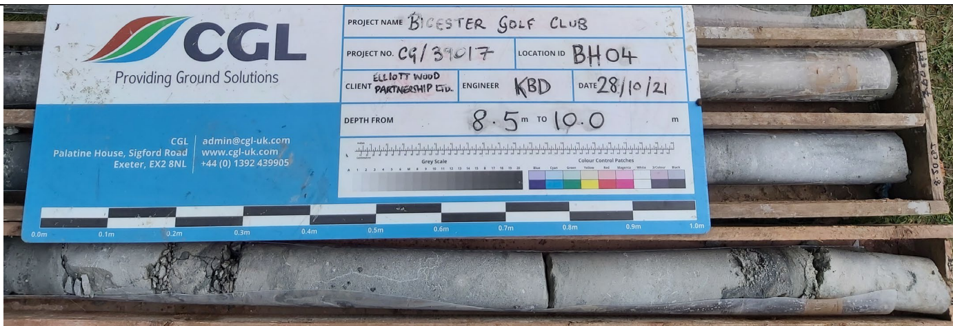
Photograph 14: Core run between 8.5 and 10.0 m bgl of mudstone of the Forest Marble Formation in BH04.
