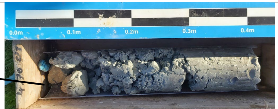
Photograph 3d: Stiff dark grey clay between 4.7 – 5.0 m bgl.
