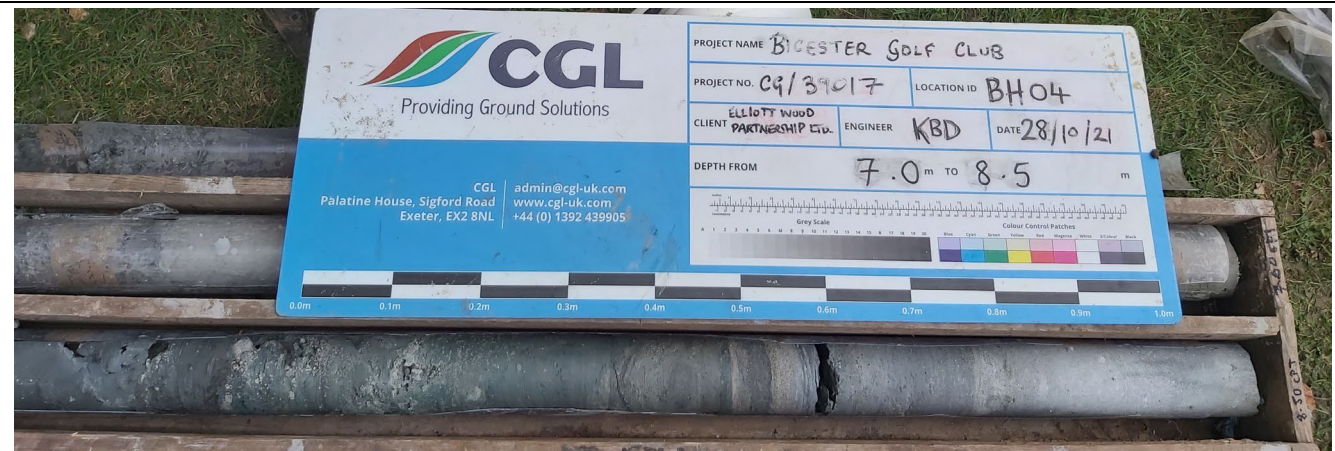
Photograph 13: Core run between 7.0 and 8.5 m bgl of mudstone, clay, and limestone of the Forest Marble Formation in BH04.
