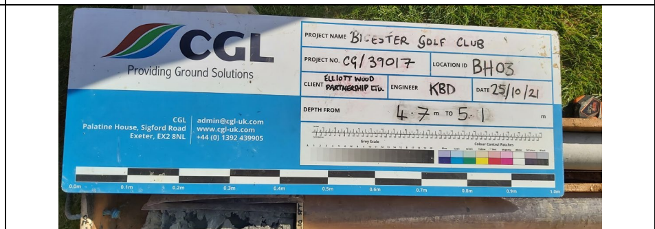
Photograph 9: Core run of dark grey mudstone between 4.70 m and 5.00 bgl.
