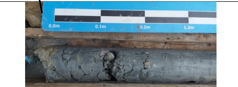
Photograph 11c: Firm slightly sandy slightly gravelly clay between 4.00 and 4.30 m bgl.
