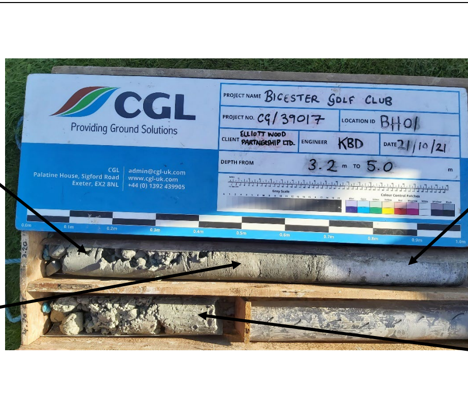
Photograph 3: Core runs between 3.2 – 4.7 and 4.7 – 5.0 in BH01
