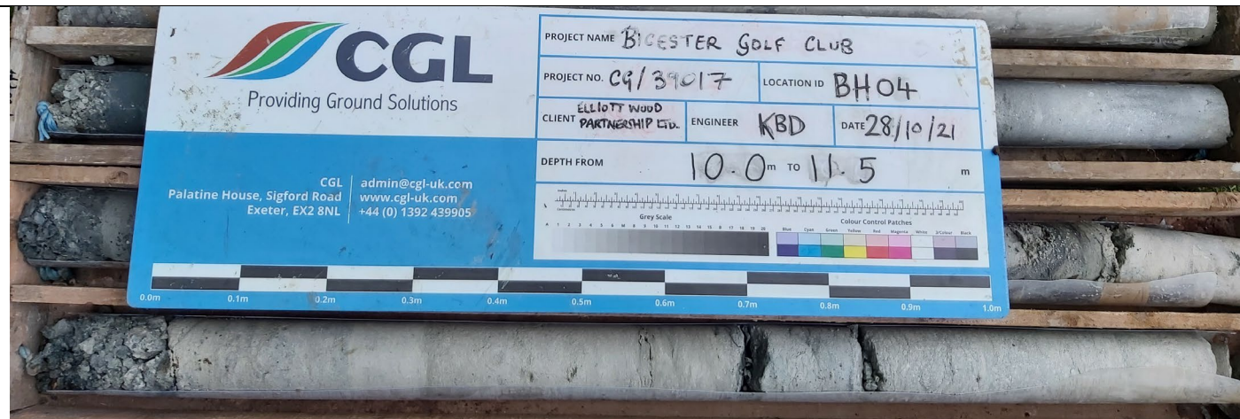
Photograph 15: Core run between 10.0 and 11.5 m bgl of mudstone of the Forest Marble Formation in BH04.
