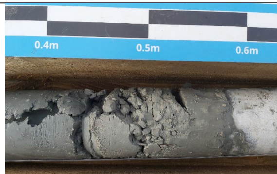
Photograph 6b: Weak mudstone recovered as gravel between 3.9 and 4.1 m bgl.
