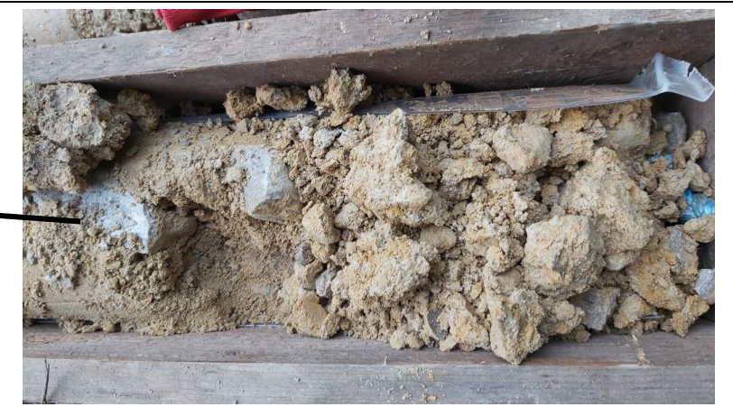
Photograph 10b: Marl when broken open. Gravel is fine to coarse sub-angular to angular grey limestone.
